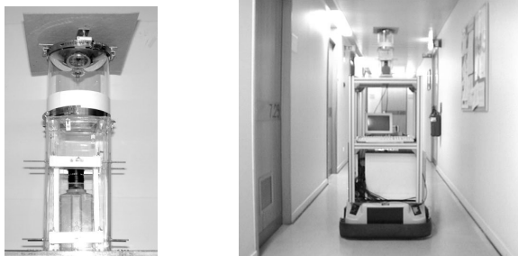
Fig. 1. Left: the omnidirectional camera. Right: the camera mounted on the mobile robot.
