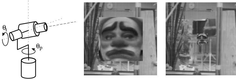
Figure 8: (left) Pan/Tilt camera. The axis of rotation are assumed to intersect in the camera optical center. (right) Simulated images with targets of scales 36% and 2.25%.
