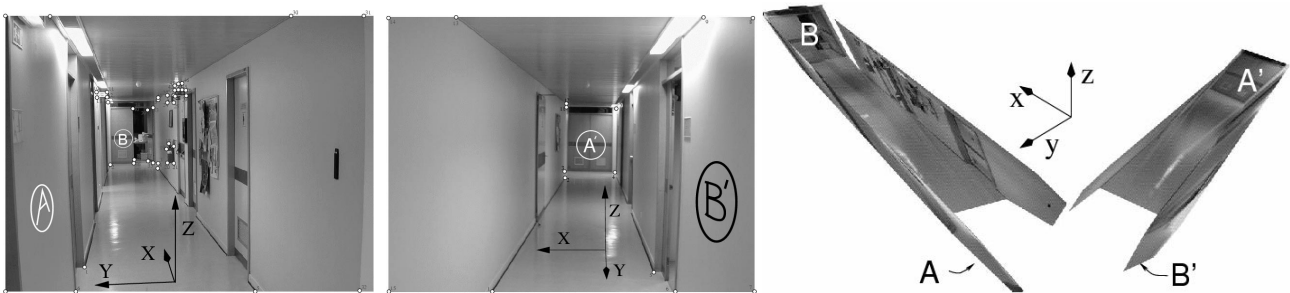
Figure 3. Left: Two indoor images. No 2D point is tracked between them Right : reconstruction.
