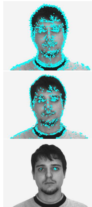
Figure 7. Example of points selected by the bottom-up saliency in the top image. In the middle image, points selected by the scale/frequency signature from the bottom-up saliency points. In the bottom image, points selected by our Gabor recognition method[8] as eye points, from the points selected by the scale/frequency signature.
