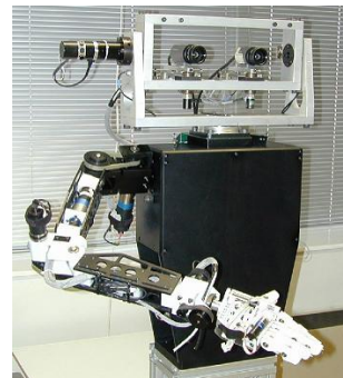
Figure 1: Baltazar. A 14 degrees of freedom humanoid torso.
