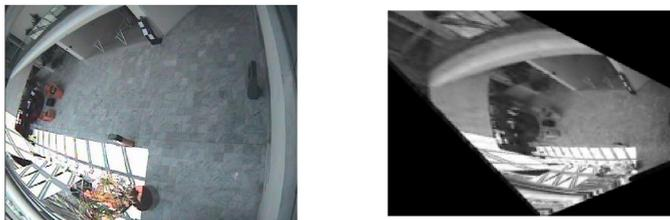
Figure 2: Original (left) and resulting transformed (right) images of the INRIA - Caviar scenario. Perspective distortion is removed by mapping the ground plane using the estimated homography.
