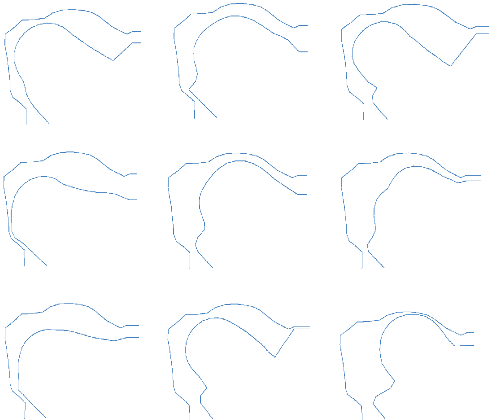
Fig. 3. Learned articulator positions for Portuguese vowels. The upper left position corresponds to the Portuguese vowel o used in for example the word só . The next position to the right corresponds to the vowel \epsilon used in sé , and the following positions corresponds to the vowels: o ( sou ), a ( vá ), e ( vê ), i ( pegar ), v ( pagar ), u ( mudo ), and i ( vi ).
