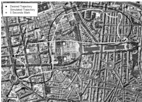
Figure 5 - Simulation: path following experiment using only the LQR controller.
