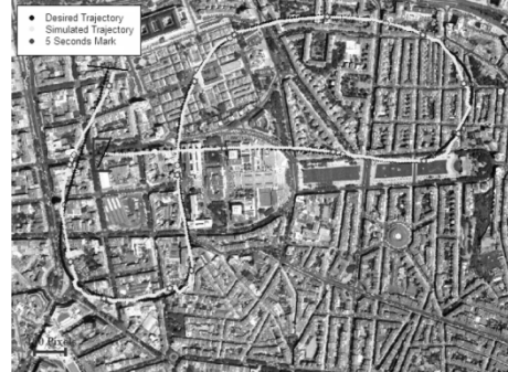
Figure 6- Simulation: path following using LQR and observer in the control.
