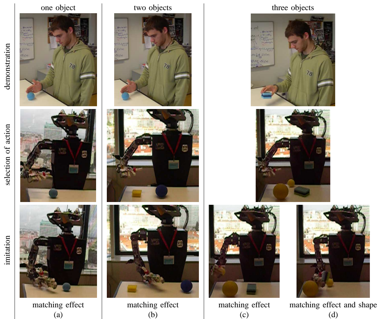
Fig. 11. Different imitation behaviors. Top: demonstration, Middle: set of potential objects, Bottom: imitation. Situation a-d represent imitation of action (a), effect (b), effect (c) and effect with shape (d).
