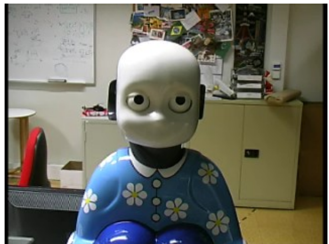
Fig. 6. Calibration procedure for the neck pan. The robot start up with significant offset in the neck pan joint, with respect to its canonical position (top). A motion of 10 degrees is applied to the neck tilt (middle). The proposed method estimates the initial pan angle and compensates it (bottom).
