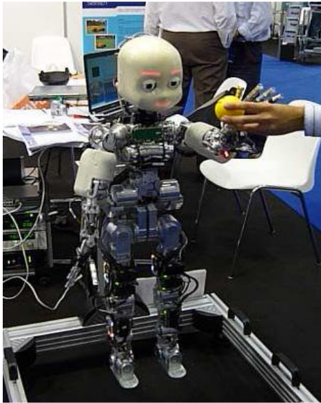
Figure 6 – The iCub robot detecting, tracking and reaching for a known object.
