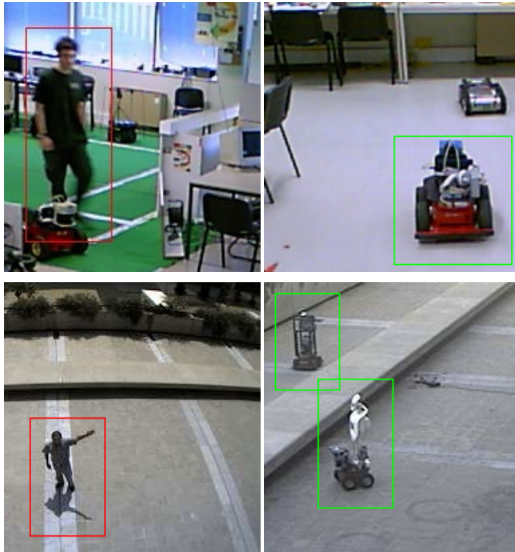
Fig. 4. Examples of person and robot training samples (on top) and real-time classification in an outdoors setting (bottom).
