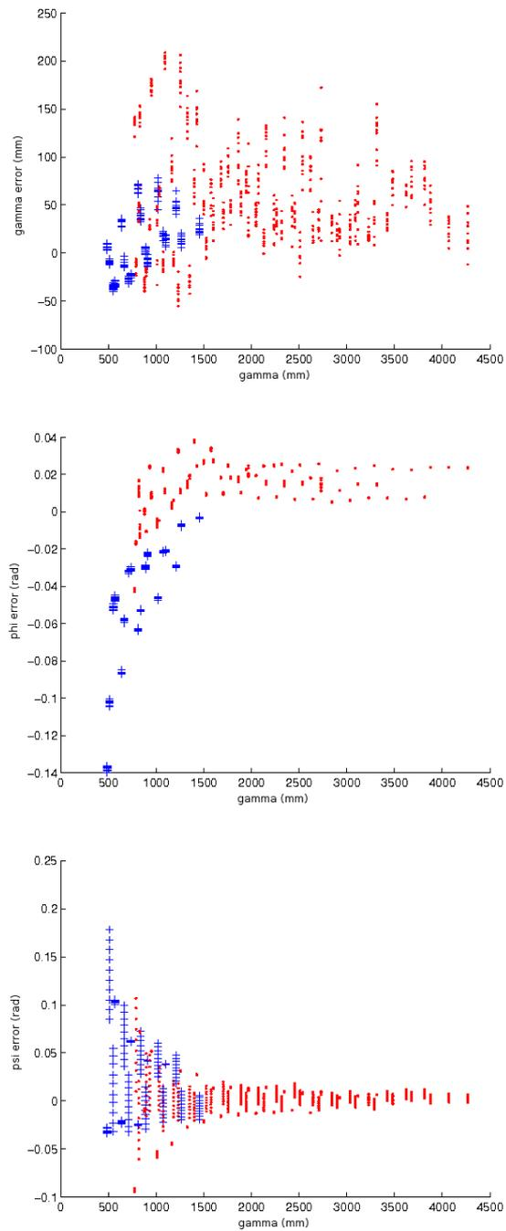
Figure 6.7:  $\gamma$ ,  $\phi$ ,  $\psi$  error for balls laying on the ground (red dots) and flying at 340mm (blue crosses).
