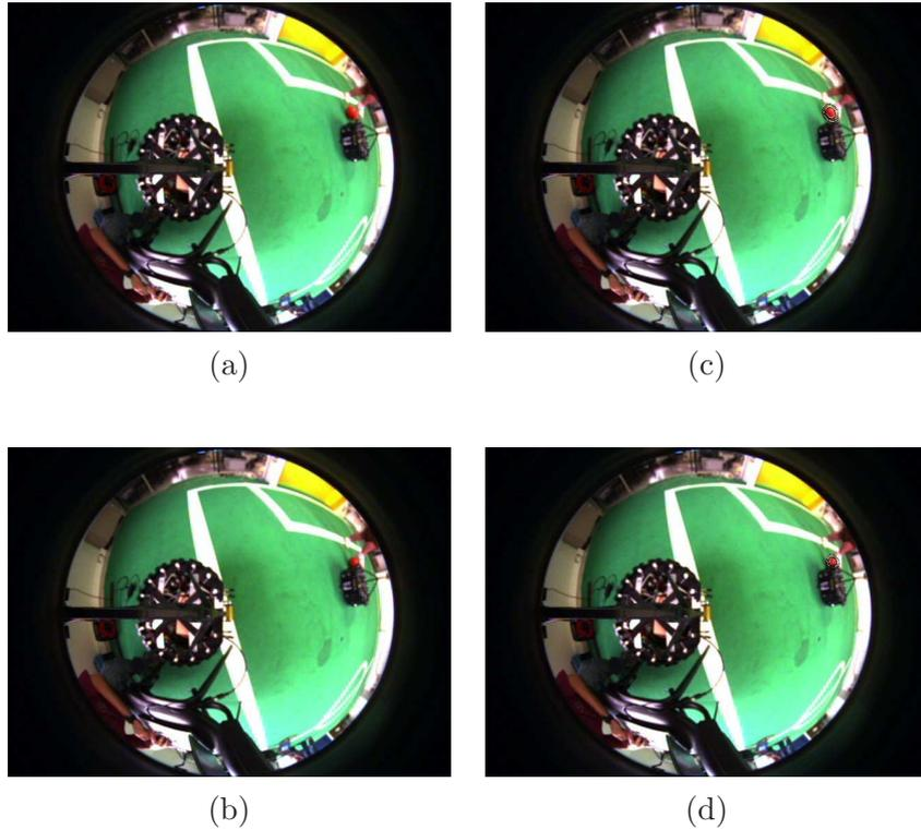
Figure 6.15: Two frames of the tracked sequence in which the ball is occluded by another robot. In the first row the ball is still fully visible, while in the second it is halfway hidden by the robot. In the first column the original images are shown, in the second one the inner and outer contours of the maximum likelihood hypothesis are drawn in white, while those of the hypothetical position corresponding to mean of all the particles, weighted by their likelihood, are drawn in black.
