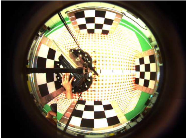
*Figure 3.5: One of the images used for calibrating the EPM model. The checkers placed at known position identify known 3D points, which are projected by the camera onto the image.*
