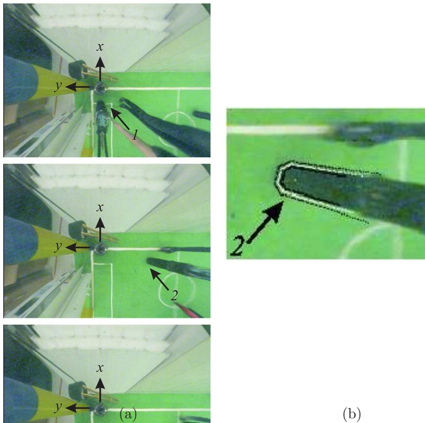
Figure 6.4: Robot tracking. Three different frames of the sequence (a) and three close-ups of the tracked robot with the contour of the best hypothesis (white) and regions used to build the color histograms (black) drawn (b).
