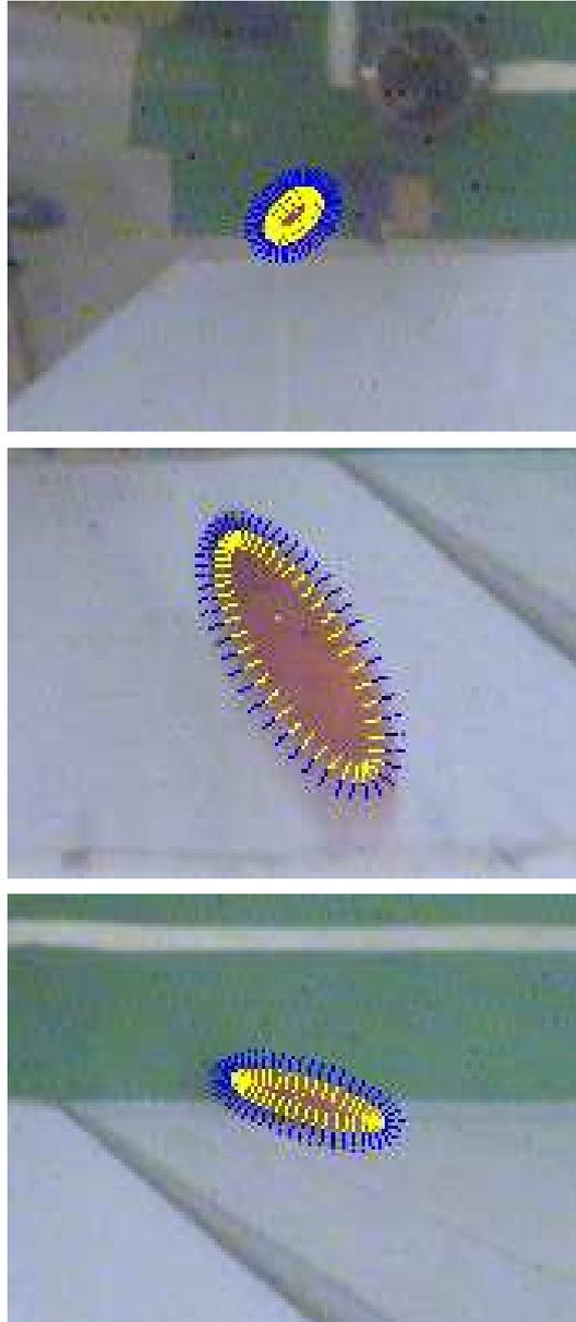
Figure 4.7: Close-up showing the pixels used to evaluate one hypothesis (one for each image), selected using B-splines. Yellow and blue pixels are used to build the inner and outer color histogram, respectively.
