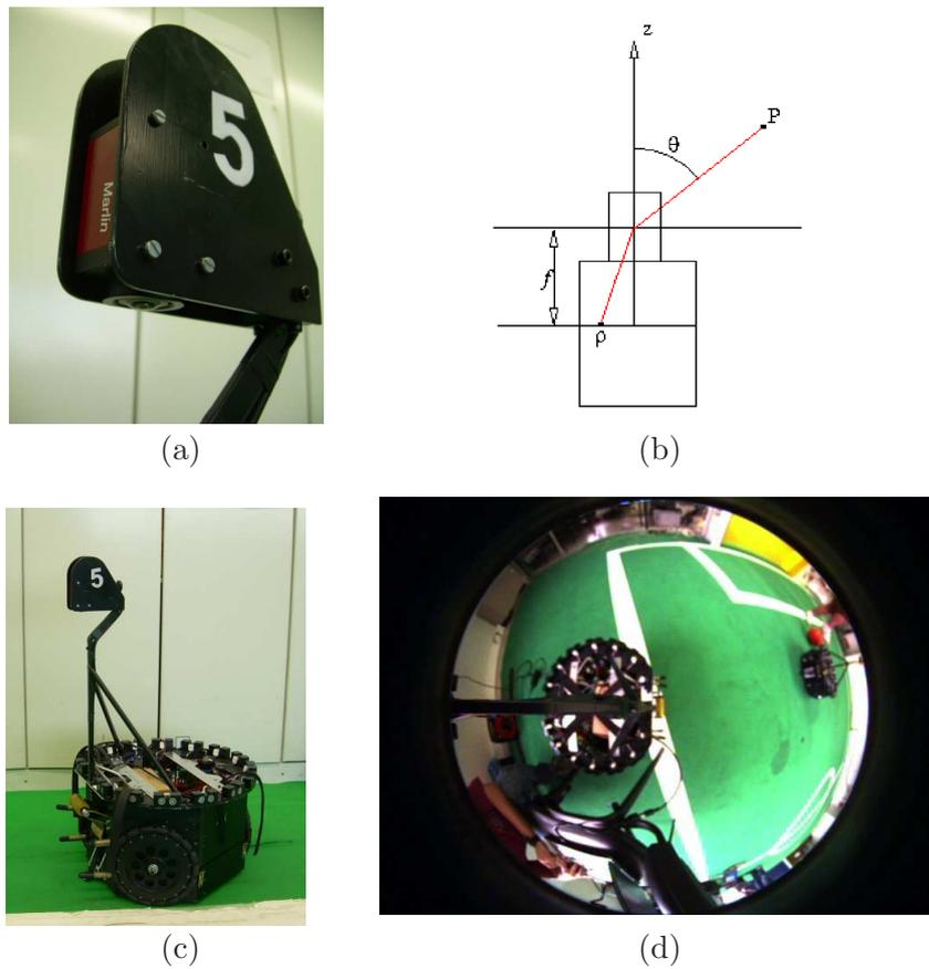
Figure 3.4: (a) Dioptric omnidirectional camera. (b) The Equidistance Projection Model. (c) The OmniSocRob robotic platform in the dioptric configuration. (d) Sample image acquired with the dioptric omnidirectional camera.
