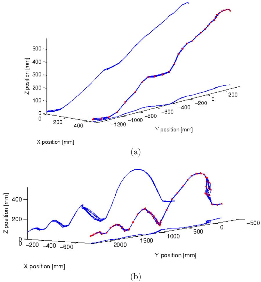
Figure 6.3: (a) Ball rolling down the ramp: plot of the tracked paths resulting from 10 runs of the algorithm performed on the same image sequence. The 10 blue lines with red points represents the 10 3D estimated trajectories of the ball, the blue lines are the projection of these trajectories on the ground and lateral plane. (b) Ball jumping: same kind of plot for the estimated trajectories of the ball in the jump image sequence.
