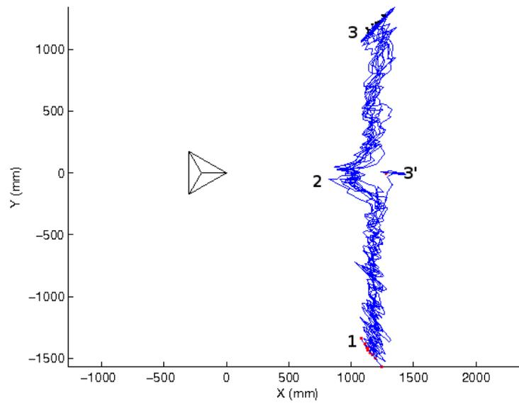
Figure 6.18: Tracked trajectories for the sequence with overlapping balls. The tracked paths start in area 1. Some inaccuracy in the localization of the tracked object can be seen in correspondence of the overlapping (2). In nine cases out of ten, the tracker followed the ball it was initialized on (ending in area 3), while in one case it switched to tracking the other ball (ending in area 3').
