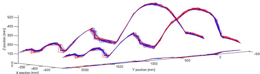
Figure 6.8: Ball jumping: plot of the tracked paths resulting from 10 runs of the algorithm performed on the same image sequence. The estimated trajectories using the PPM and the UPM models are shown, respectively, with blue and red lines. Both the 3D trajectory and its projections on the ground and lateral planes are shown.
