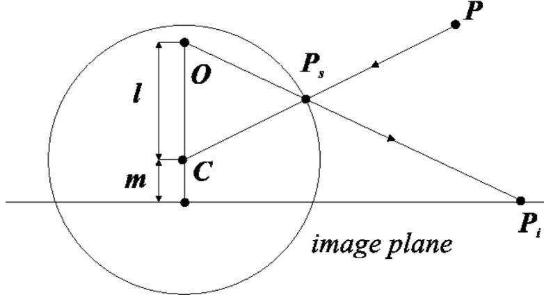
Figure 3.2: The Unified Projection Model.
