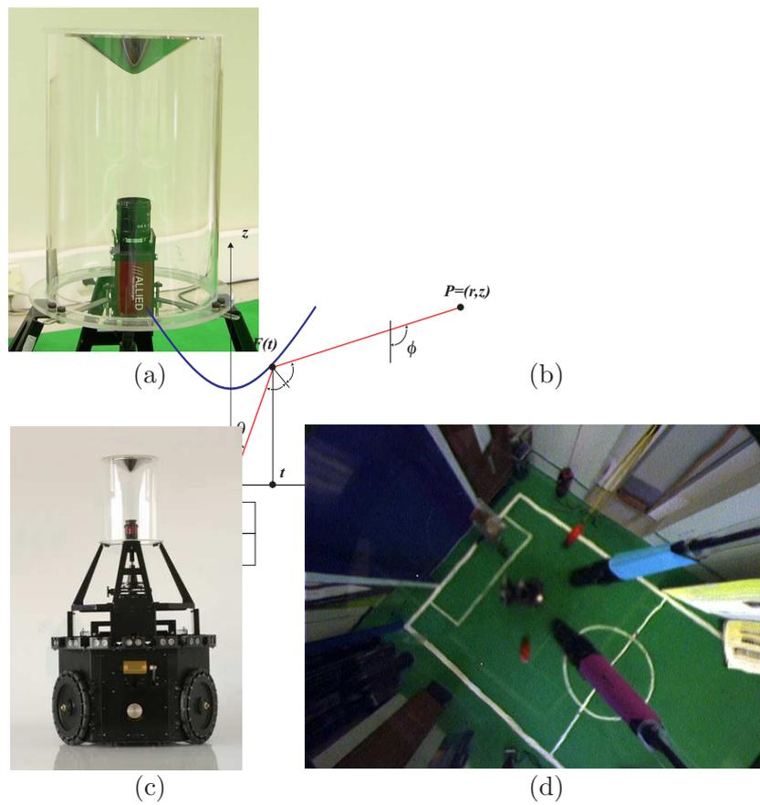
Figure 3.1: (a) Catadioptric omnidirectional camera. (b) The generic Catadioptric Projection Model. (c) The OmniSocRob robotic platform in the catadioptric configuration. (d) Sample image taken with the catadioptric omnidirectional camera in a RoboCup MSL scenario.
