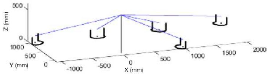
Figure 4.4: Plot of the 3D points projected to obtain the 2D contour points for robots at different positions. Again, the black line connects the projection center to the ground plane.
