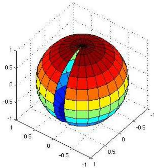
Figure 4.2: Polygonal model of a sphere (some of the faces have been removed for visualization).
