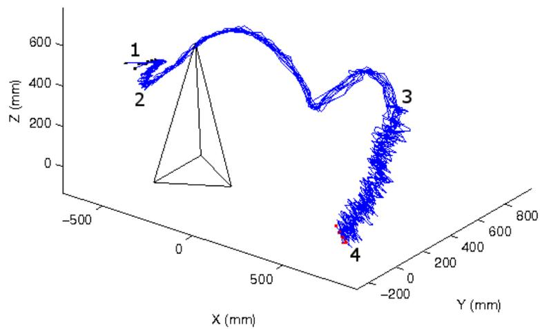
Figure 6.12: Ball jumping: plot of the tracked paths resulting from 10 runs of the algorithm performed on the same image sequence. The pyramid represents the robot acquiring the image sequence. The tracked paths start in 1. At first, the ball is held by a person who lowers it (tracks from area 1 to 2), then the ball is thrown in the air, bounces on the floor and then bounces on the floor and off the wall at the same time (3). The tracked paths end in 4.
