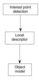
Figure 1.2: Main steps of component-based object recognition.
