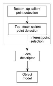
Figure 1.3: Architecture of our component-based object recognition approach
