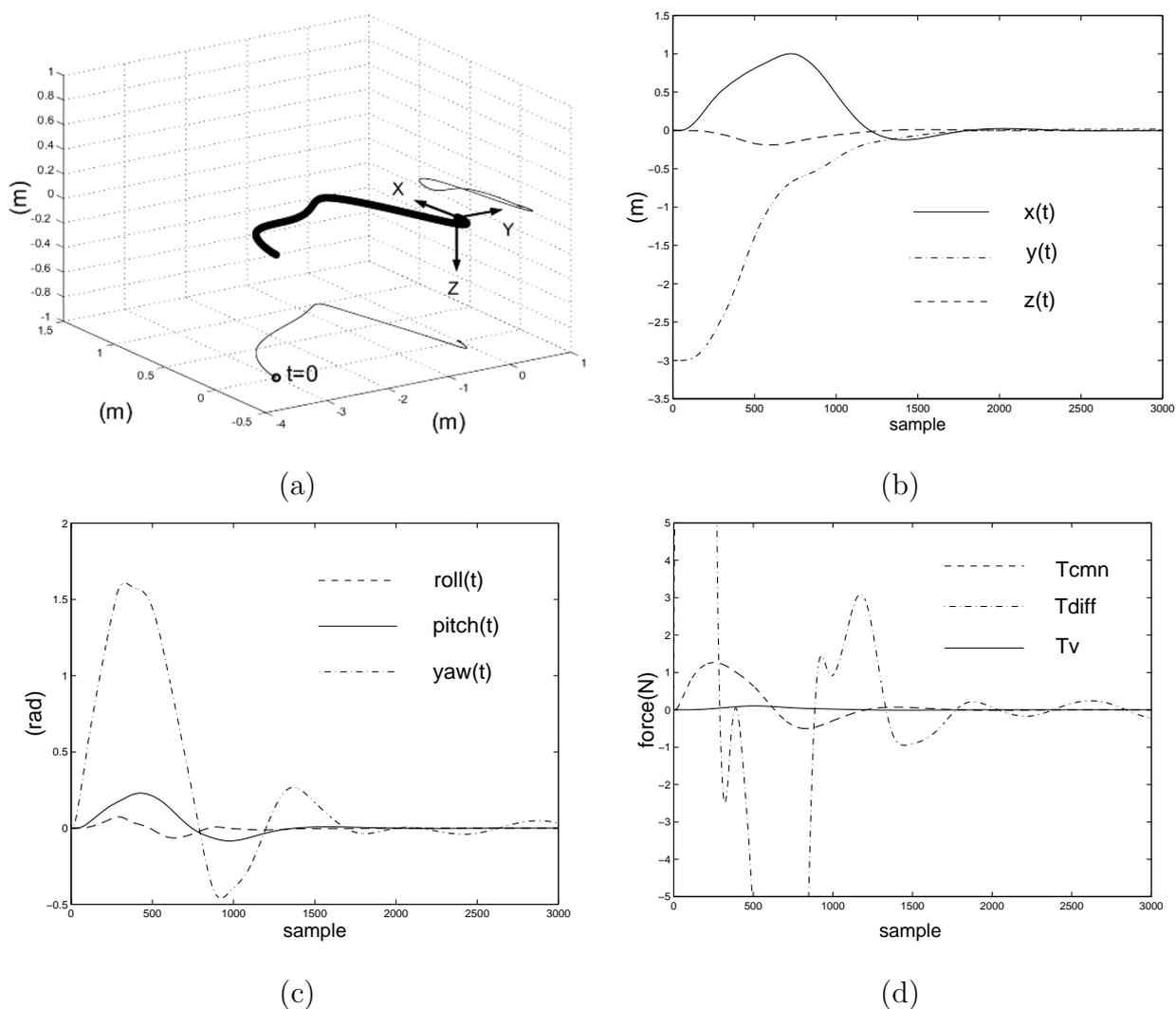
Figure 6.1: Simulation results of a station keeping test with the simulation model; (a) vehicle under closed-loop control while recovering an initial lateral deviation; projections of the trajectory onto the horizontal and vertical plane are shown together with the earth-fixed reference frame ; (b) position over time; (c) orientation over time; (d) generated control signals.
