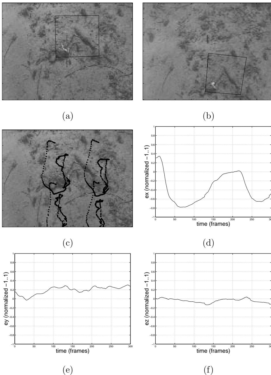
Figure 6.4: Image based control for position, orientation and altitude of the ROV; (a) initial selected landmark; (b) landmark at the end of the recording phase; (c) temporal trajectory of the window corner coordinates; (d) positional offset along the image x-axis; (e) positional offset along the image y-axis; (f) error in window area.
