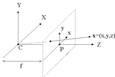
Figure 2.3: The pinhole camera model
