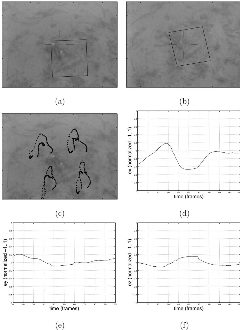
Figure 6.3: Point-to-point positioning with ROV at open sea; (a) initially selected landmark; (b) landmark position in image at the end of the experiment; (c) trajectory of the window corners during the trial; (d) positional offset along the image x-axis; (e) positional offset along the image y-axis; (f) error in window area.
