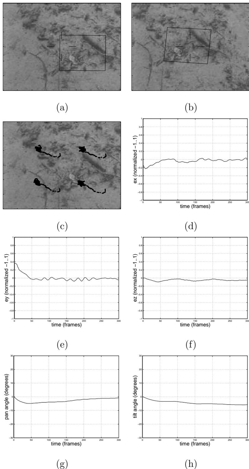
Figure 6.6: Image based control for position, orientation and altitude of ROV at open sea, with image stabilization; (a) initial selected landmark; (b) landmark at the end of the recording phase; (c) temporal trajectory of the window corner coordinates; (d) positional offset along the image x-axis; (e) positional offset along the image y-axis; (f) error in window area; (g) temporal evolution of the pan angle; (h) temporal evolution of the tilt angle.
