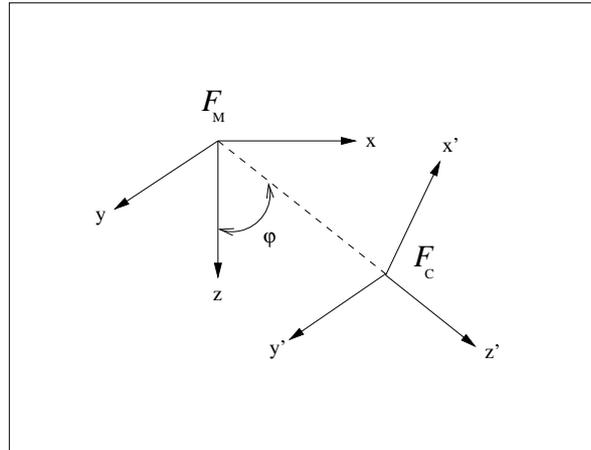
Figure 4.7: Position and orientation of the camera frame,  $\mathcal{F}_C$ , in the vehicle reference frame,  $\mathcal{F}_M$ .
