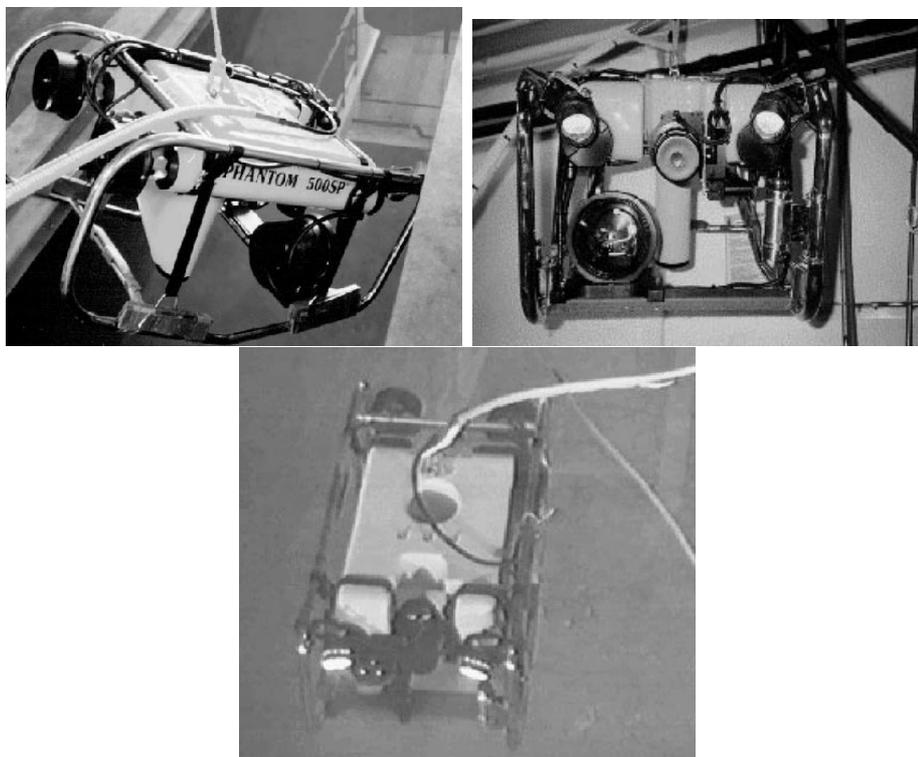
Figure 4.3: Remote operated underwater robot with on-board pan- and tilt-camera.
