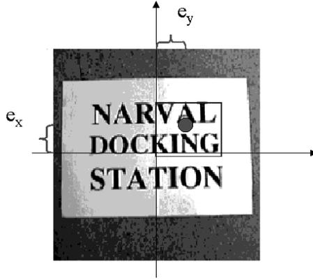
Figure 5.5: Point-to-point positioning by driving the centroid of the tracked window to the image center.
