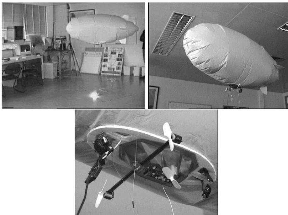
Figure 4.1: Radio controlled indoor blimp with on-board camera.
