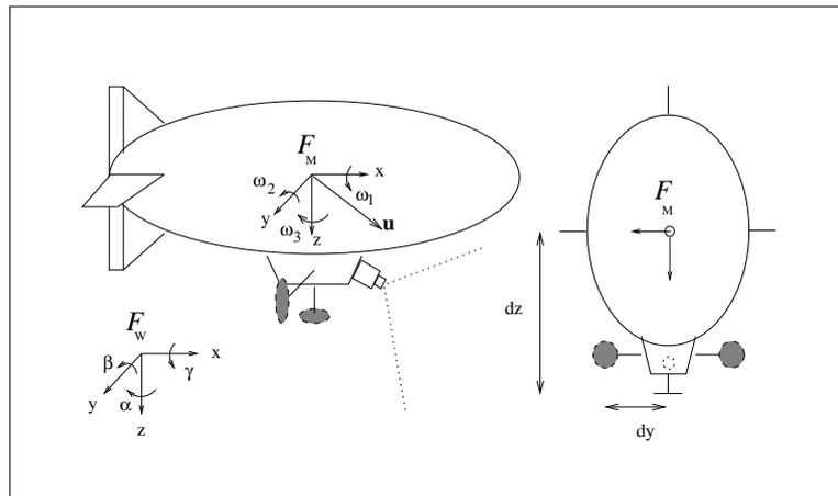
Figure 4.5: Definition of reference frames.
