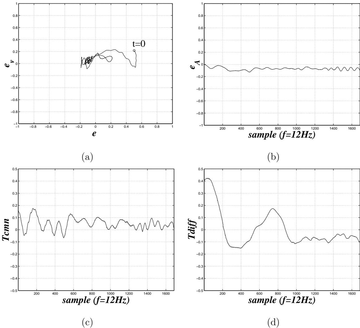
Figure 6.2: Docking and station keeping test with the blimp. (a) trajectory of the centroid of the tracked window (image errors in normalized pixel coordinates); (b) difference between the area of the image patch and the tracked window; (c) common mode forward velocity control; (d) differential angular velocity control.
