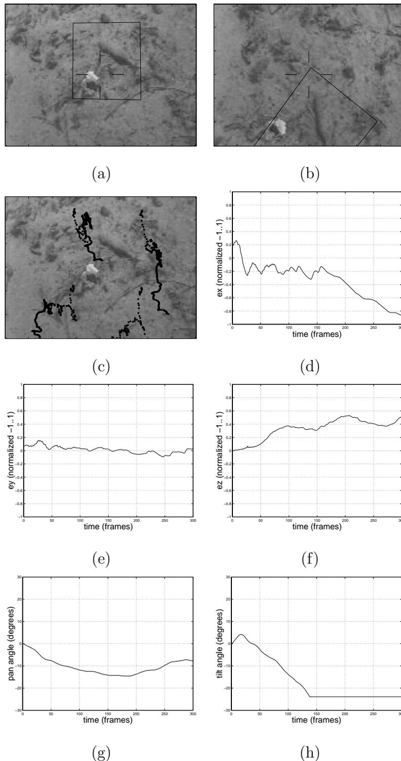
Figure 6.5: Image stabilization with pan and tilt unit for the ROV onboard camera at open sea; (a) initial selected landmark; (b) landmark at the end of the recording phase; (c) temporal trajectory of the window corner coordinates; (d) positional offset along the image x-axis; (e) positional offset along the image y-axis; (f) error in window area; (g) temporal evolution of the pan angle; (h) temporal evolution of the tilt angle.
