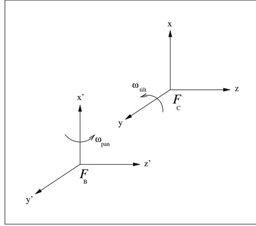
Figure 4.6: Schematics of a pan and tilt camera;  $\mathcal{F}_B$  base frame in which the pan angle is defined;  $\mathcal{F}_C$  camera reference frame in which the tilt angle is defined.
