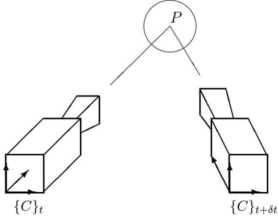
**Figure 2.6:** Camera in motion and the related coordinate frames.
