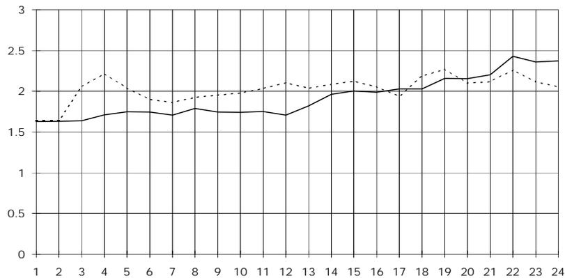
**Figure 3.18:** The average between the left and right flows obtained in an experiment with (dotted line) and without (filled line) velocity control. The nominal flow is 2.0 pixels/frame and the nominal velocity 80mm/s.
