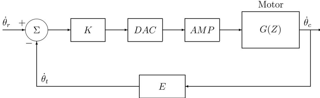
**Figure 6.8:** The control system block diagram when operating in Proportional Velocity mode.
