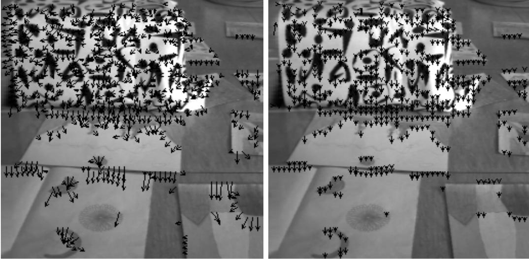
**Figure 4.7:** The left image shows a sample of the normal flow field measured during the robot motion. The right image shows the resulting inverse projected flow, where the obstacle can be easily detected.
