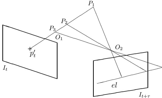
**Figure 2.3:** The epipolar line,  $el$ , is the locus of all the corresponding points of  $p'_t$  when depth ranges from zero to infinity.
