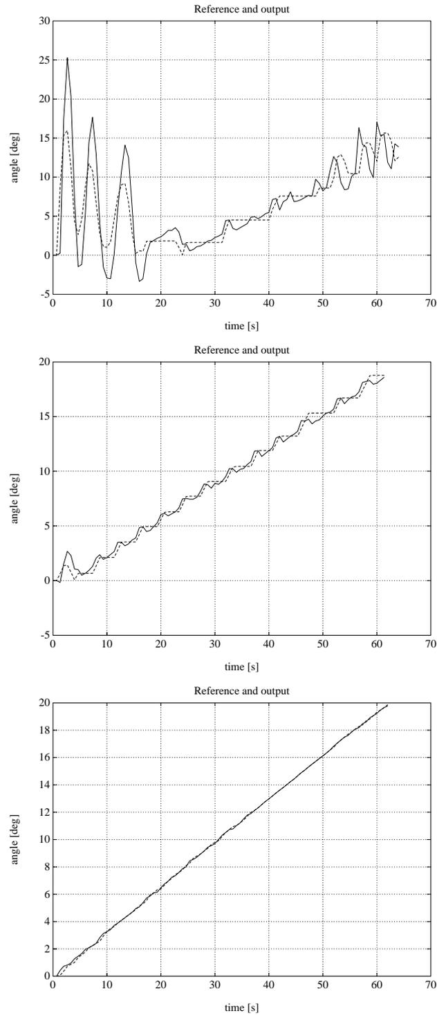
**Figure 6.14:** Tracking trajectories. From the first experiment to the second, we have doubled the sampling period, thus halving the minimum detectable speed to  $1.5^{\circ}/s$ . On the final experiment, the control strategy combines smooth pursuit and microsaccadic movements.
