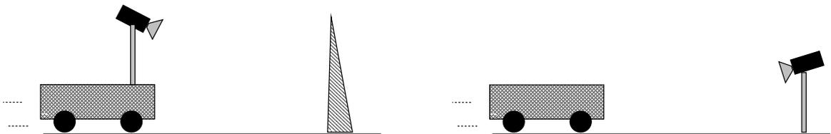
**Figure 5.1:** The left diagram shows the *ego-docking* where a robot, equipped with a camera and computing resources, docks to a specified surface. Instead, in the *eco-docking*, shown on the right, the camera is attached to a single docking station which may serve multiple robots.
