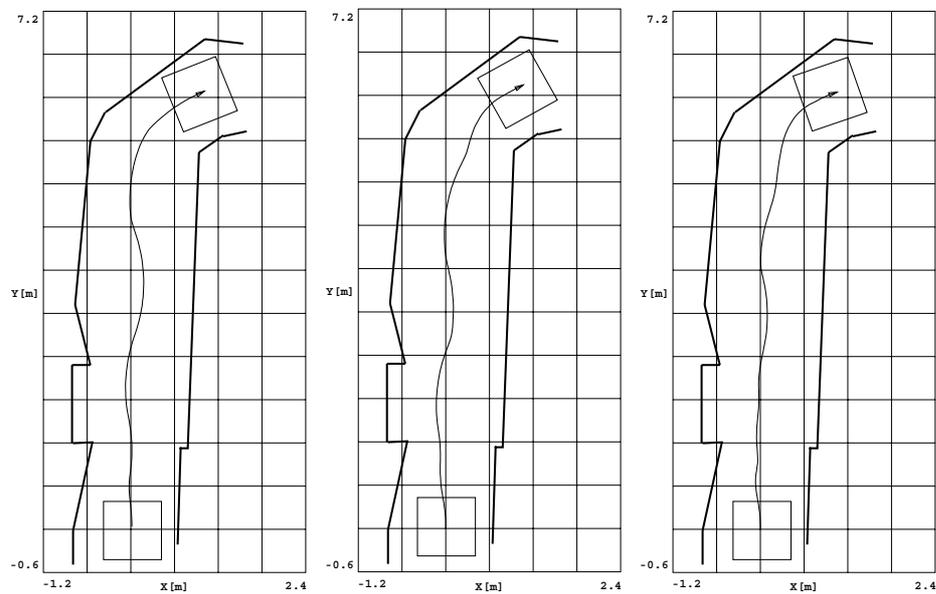
**Figure 3.17:** Corridor experiment. The proportional gain is fixed in  $K_p = 1.4$ , while the derivative gain increases from left to right  $K_d = 1.0, 1.2, 1.4$ .
