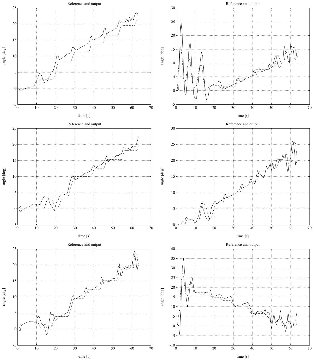
**Figure 6.13:** On the left column (experiments i, ii and iii), we see the effect of increasing the proportional gain of the gaze controller. On the right column, (experiments iv, v and vi) we start by adding some integrative action, then some derivative action, and finally remove the integral action.
