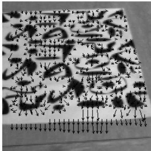
**Figure 5.7:** Sample of the normal flow field used to estimate the affine motion parameters.
