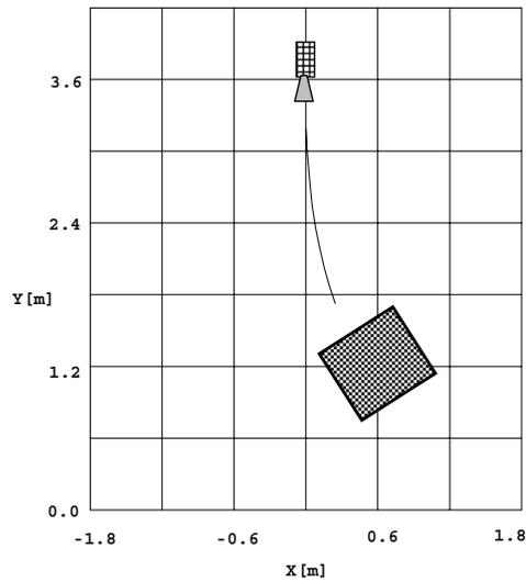
**Figure 5.10:** Trajectory during the *ego-docking* manoeuvre to a static docking station. The trajectory is recovered using odometry.
