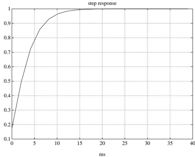
**Figure 6.7:** Simulated step response for the vergence motor.
