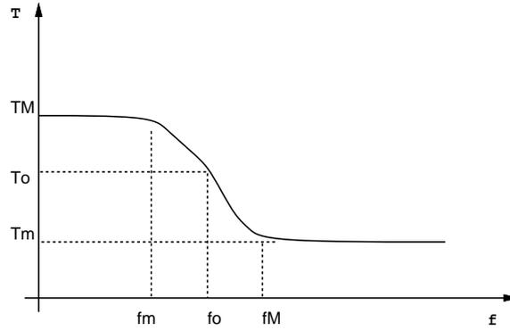
**Figure 3.9:** The sigmoid function, used in the velocity control loop, describes how the robot forward speed should change, with relation to the measured flow. It is used to introduce a smooth saturation on the robot velocity.
