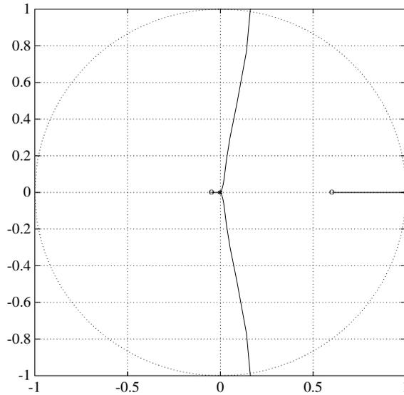
**Figure 3.7:** Root-Locus corresponding to the proportional-derivative controller. The derivative gain was fixed at  $K_d = 1.5$ .
