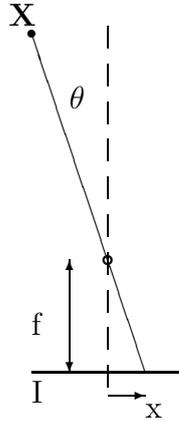
**Figure 6.10:** Simplified kinematics. The relationship between the target position in the image and its angular position, with respect to the vergence and tilt joints.
