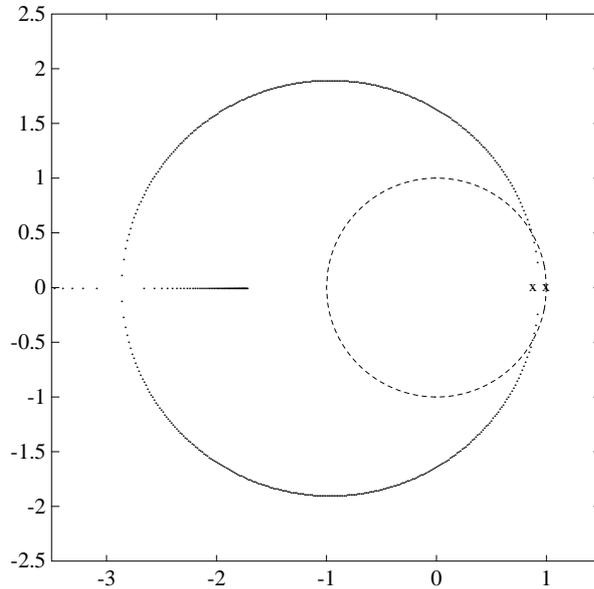
**Figure 6.5:** Root Locus of uncompensated system for vergence. The unit circle is shown in dotted line. The system becomes unstable with a proportional controller.
