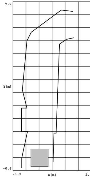
**Figure 3.15:** Setup used for the corridor experiment. The corridor is just slightly larger than the robot, and has a tight turn in the end.
