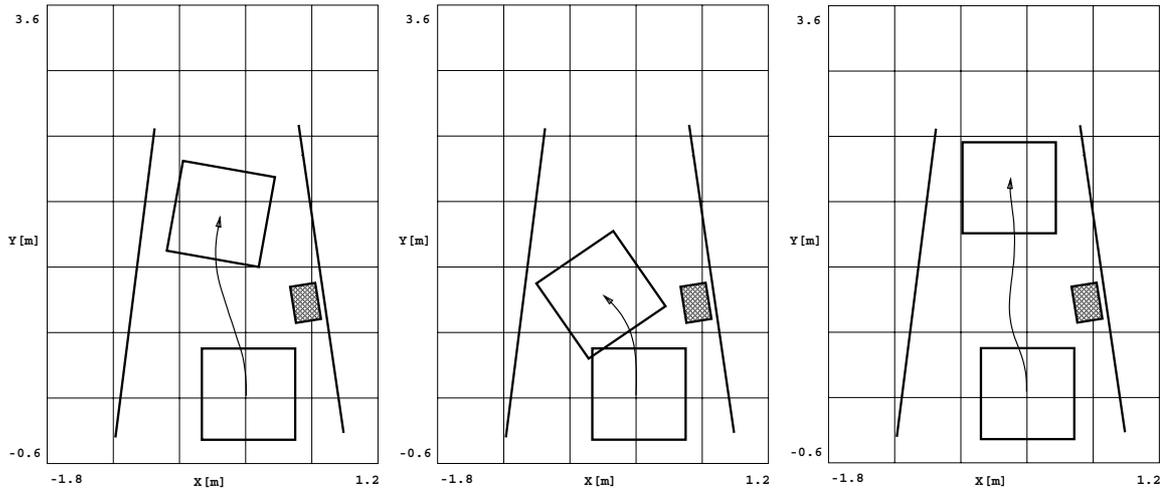
**Figure 3.14:** Funneled corridor experiment. The leftmost and rightmost plots show the results of increasing the proportional gain while decreasing the derivative gain. In the center, it is seen the unstable behaviour due to the insertion of the integral action.
