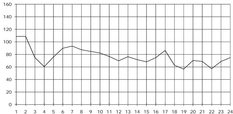
**Figure 3.19:** The robot speed in mm/s during the funneled corridor experiment. As the corridor narrows, also the velocity decreases for safer operation.
