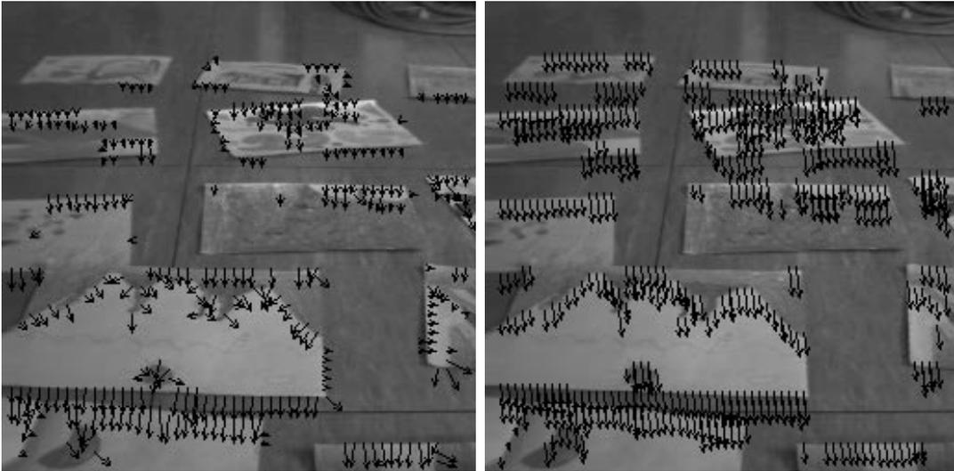
**Figure 4.6:** The left image shows a sample of the ground plane normal flow field measured during the robot motion. The right image shows the flow field that results from the inverse projection.
