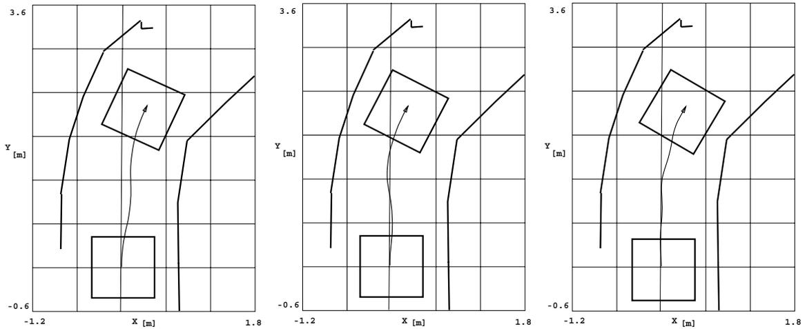
**Figure 3.11:** Results obtained in the closed loop operation in the turn experiment. The controller settings were  $K_p = 1.5$ ,  $K_i = 0$  and using for  $K_d$  the values (from left to right) of 1.0, 1.2 and 1.4. The trajectory was recovered using odometry.
