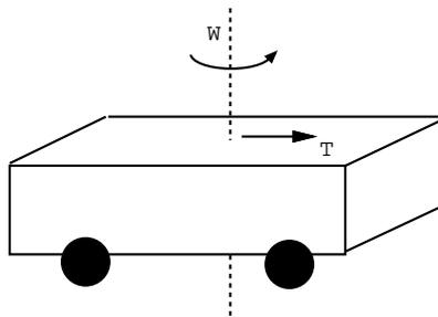
**Figure 5.2:** Mobile platform motion degrees of freedom.
