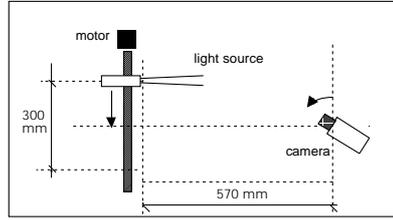
**Figure 6.12:** Experimental setup for the gaze control system.
