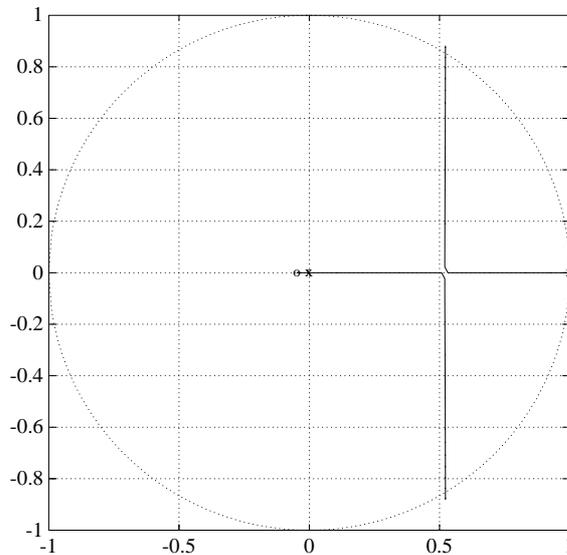
**Figure 3.6:** Root-Locus corresponding to the proportional controller. The unit circle is shown in dotted line for easier stability analysis.
