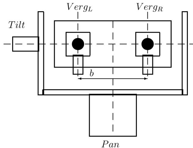
**Figure 6.1:** Schematic representation of the stereo head. The degrees of freedom are two independent vergences and common tilt and pan. The baseline, *b*, can be manually adjusted.
