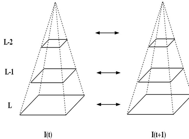
**Figure 2.5:** Coarse-to-fine control strategy based on a Gaussian pyramid.
