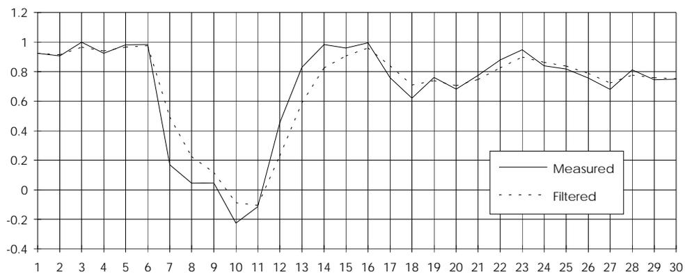
**Figure 3.3:** Difference between the left and right average flows, during the obstacle detection experiment. The full path takes 20 seconds, covering a distance of about 2.4m. The filtered signal (dashed line) results from applying a first order filter to the measured values.
