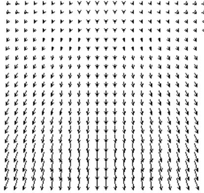
**Figure 4.3:** Flow field generated for the simulation study, which corresponds to a robot moving forward on a flat ground, with a camera pointing down.
