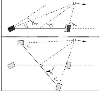
**Figure 6.11:** Fast movement (saccadic type) of the pan motor, followed by the appropriate vergence compensation.
