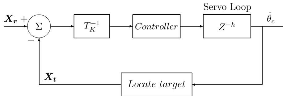
**Figure 6.9:** Gaze control loop. At the sampling rate of the visual feedback loop, the inner servo loops can be considered as simple delays.
