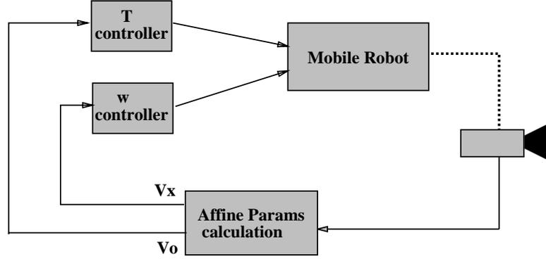
**Figure 5.5:** Structure of the overall heading and docking speed control system.
