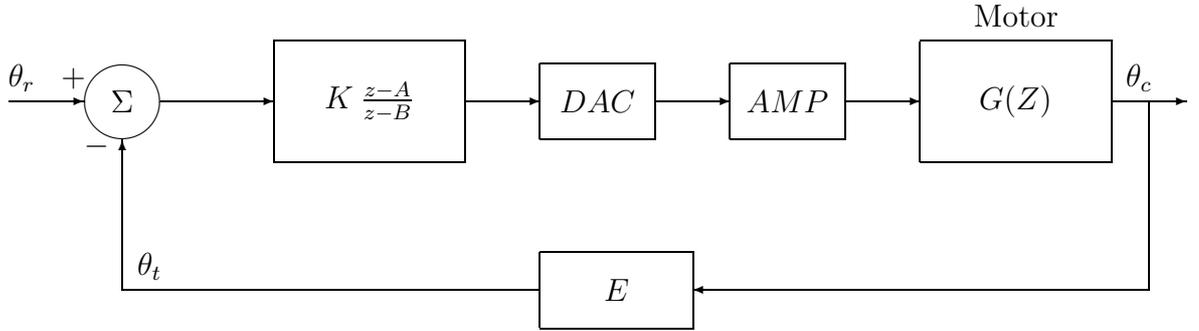
**Figure 6.4:** Block diagram of the complete system in position control mode.
