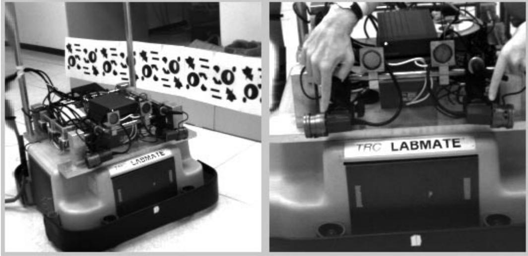
**Figure 3.1:** Robee with the divergent stereo camera setup
