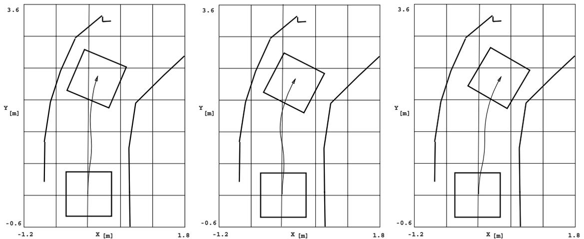
**Figure 3.12:** Results obtained in the turn experiment (closed loop operation). The controller settings were  $K_d = 1.2$ ,  $K_i = 0$  and using for  $K_p$  the values (from left to right) of 1.25, 1.5 and 1.75. The trajectory was recovered using odometry.
