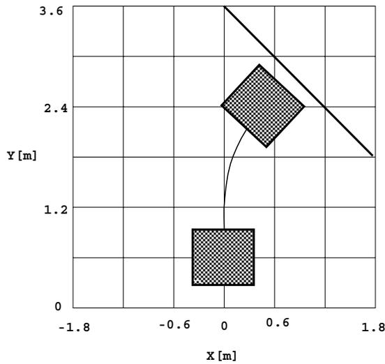
**Figure 5.8:** Trajectory during a real *ego-docking* manoeuvre. The trajectory is recovered using odometry.
