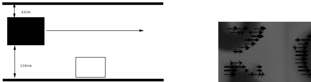
**Figure 3.2:** Experimental setup for the obstacle detection experiment. A sample of the computed optical flow is shown on the right.
