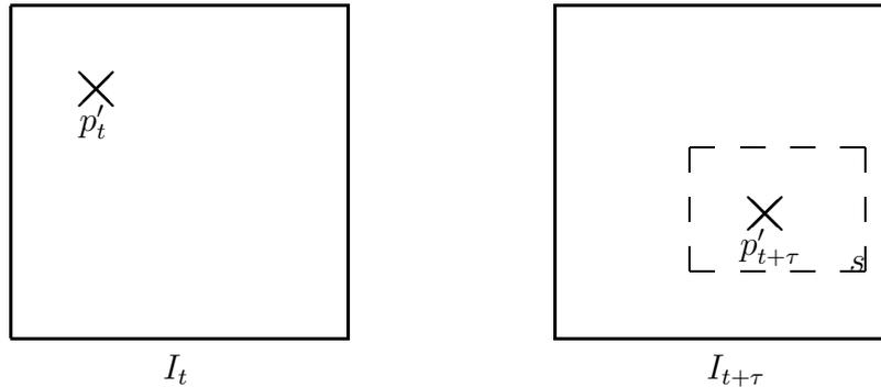
**Figure 2.2:** The problem of correspondence search in a stereo pair. To determine the point  $p'_t + \tau$ , correspondent to  $p'_t$ , the area  $S$  has to be searched.
