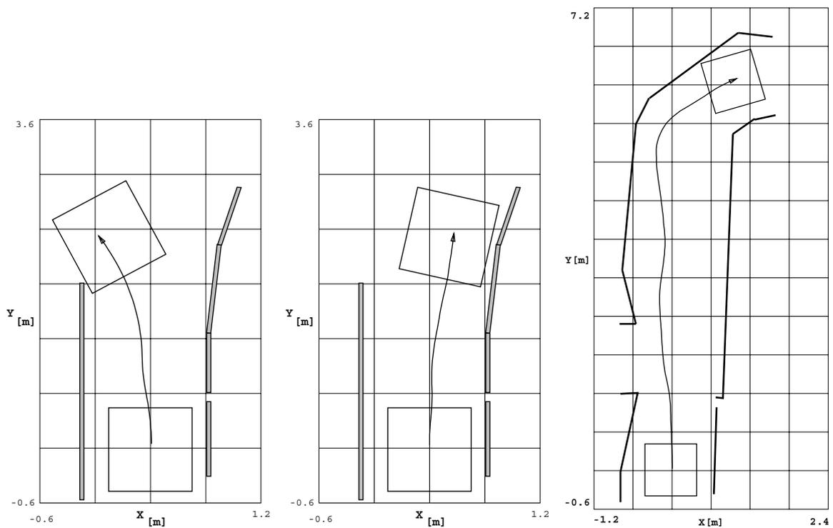
**Figure 3.20:** Sustained mechanism experiment. The left diagram corresponds to the behaviour of the robot without the sustaining mechanism. At the center, due to the sustaining behaviour, the robot manages to follow the right wall. The rightmost diagram corresponds to an experiment along the corridor with an open door on the left and a lack of texture on the right.
