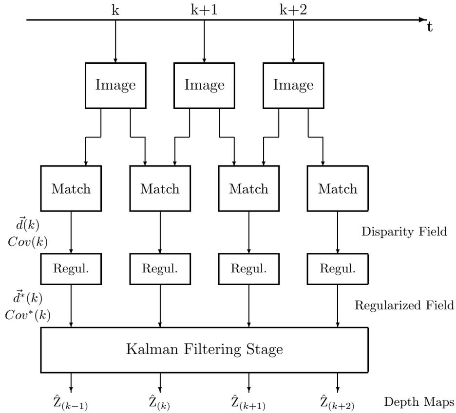
**Figure 2.8:** Block diagram of the 3D vision system.
