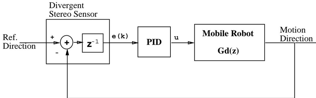
**Figure 3.5:** This block diagram illustrates a simple modelization of the robot navigation system
