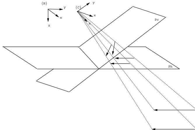
**Figure 4.4:** Inverse perspective mapping. The coordinate systems (C) and (H) share the same origin even though in the picture they have been drawn separately for the sake of clarity. While on (C) the motion of the ground floor is perceived as a complex vectorial pattern, in (H) all the vectors have equal length and orientation under translational motion.
