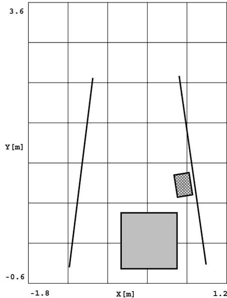
**Figure 3.13:** Setup used for the funneled corridor experiment. In this scenario, the robot has to avoid an obstacle while managing to keep the track in the funneled corridor.
