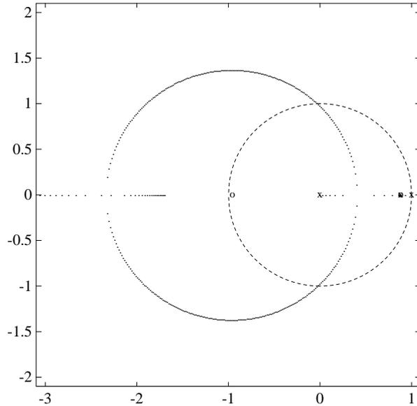
**Figure 6.6:** Root Locus of PD compensated system for vergence. The unit circle is shown in dotted line.
