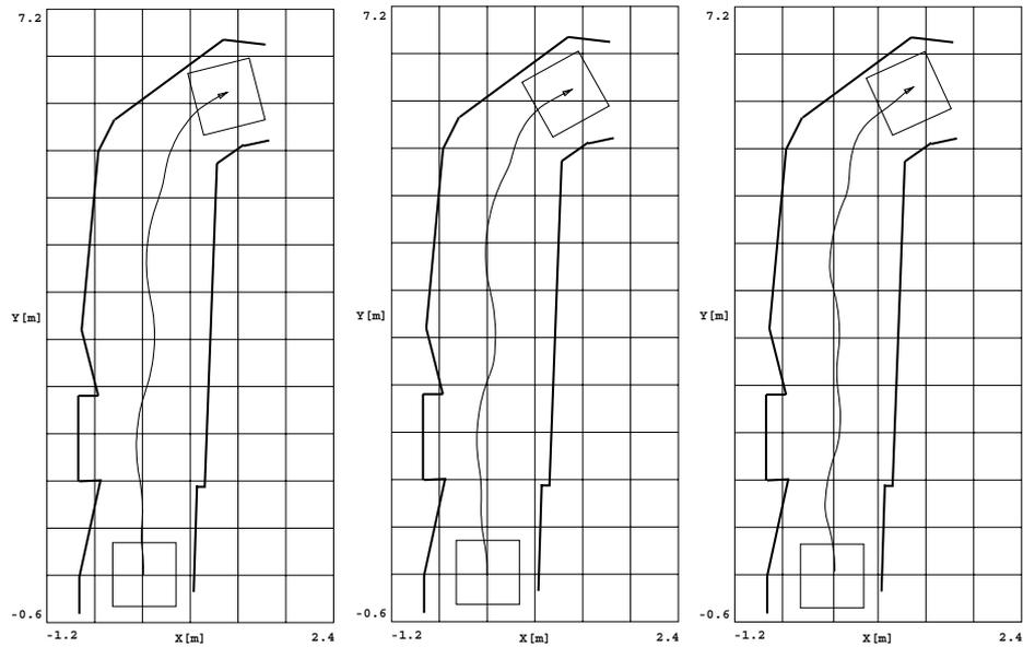
**Figure 3.16:** Corridor experiment. The derivative gain is fixed in  $K_d = 1.2$ , while the proportional gain increases from left to right  $K_p = 1.2, 1.4, 1.6$ . The integral gain is not used.
