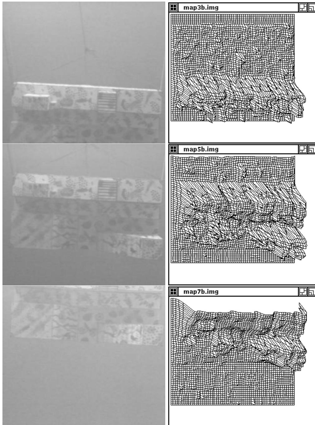
**Figure 2.11:** The left column shows the input image sequence, acquired during the camera motion in the experimental pool. On the left side, the perspective view of the reconstructed depth maps are shown.
