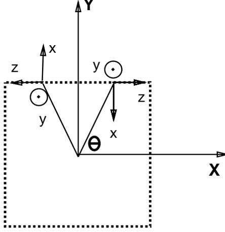
**Figure 3.4:** Coordinate systems associated to the vehicle for the analysis of the rotational motion.
