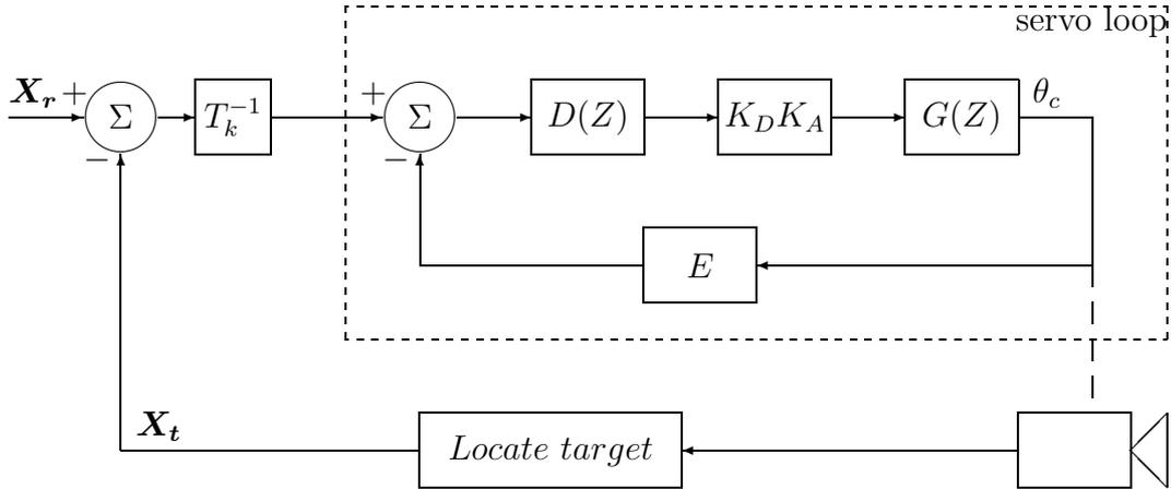
**Figure 6.3:** Complete loop for gaze control. This figure shows the cycle of image acquisition, locating the target and generating new motor commands to keep the object centered in the retina.
