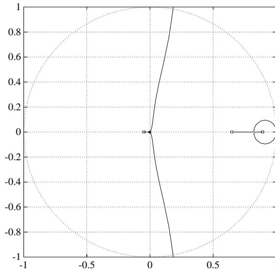
**Figure 3.8:** Root-Locus corresponding to the PID controller.
