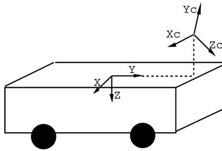
**Figure 5.3:** Sensor and motor coordinate frames.
