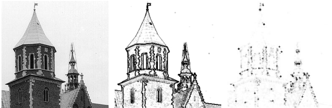
Figure 4.1: Feature Selection: original image (left), sum of the squared derivatives (center), smallest eigenvalue of G with features marked (right)
