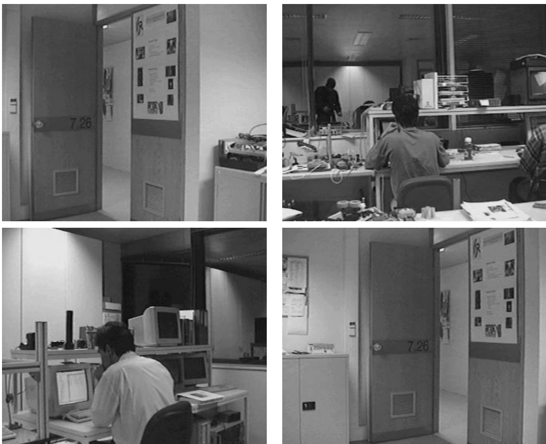
Figure C.8: The VisLab sequence was recorded by a camera on top of a tripod and rotating around the vertical axis, thus inducing simple sideways image motion. It contains 84 images of 336 \times 276 pixels.
