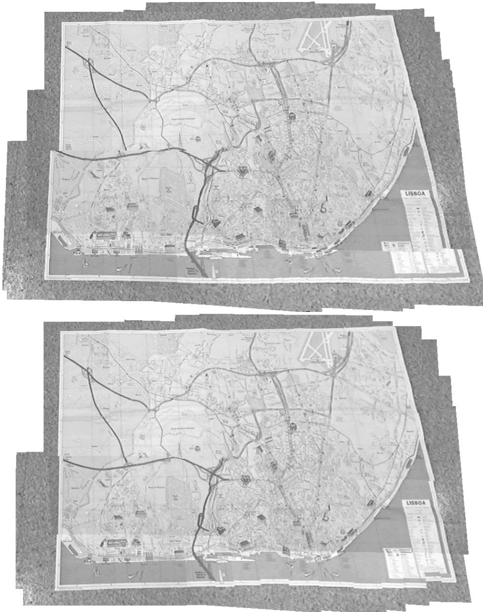
Figure 4.8: Example of direct mosaic registration. The top mosaic was created using the frame-to-frame motion estimation whereas direct mosaic registration was used for the lower one.
