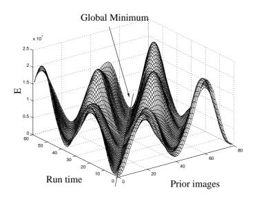
**Fig. 4.3**: A 3D plot of images acquired at run time, R versus those acquired *a priori*, P. This plot represents the traversal of a single corridor. The global minimum is the estimate of the robot's topological position.
