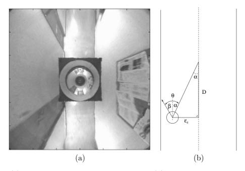
**Fig. 4.4**: (a) A bird's-eye view of the corridor and (b) the measurements used in the control law: the robot heading,  $\beta$ , the distance,  $\epsilon_d$  to the corridor centre, and the angle,  $\alpha$  towards a point ahead in the corridor central path. The error used for controlling the robot orientation is  $\theta$ .
