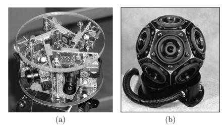
**Fig. 1.2**: Camera-only omnidirectional systems: (a) The RingCam uses board cameras mounted in pentagonal fashion. (b) Very large resolution images are obtained using the Dodeca camera.
