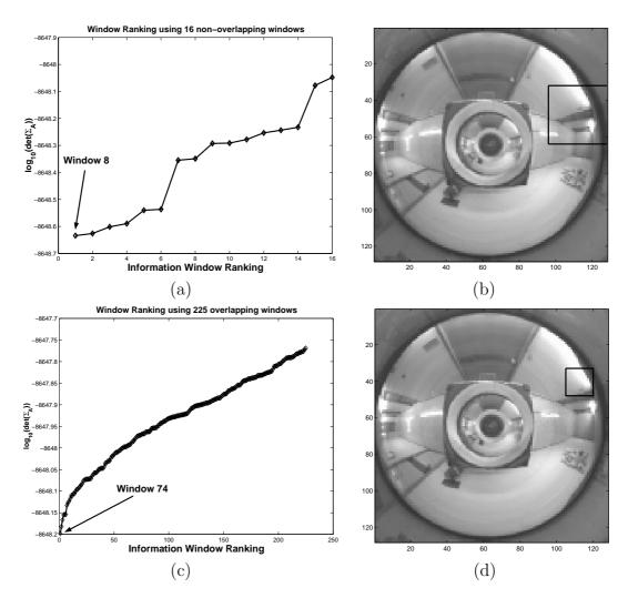
**Fig. 5.6**: Graphs of the information contained in each Information Window versus the window rank using (a) non-overlapping and (c) overlapping windows. The best (b) non-overlapping and (d) overlapping Information Window in an image.
