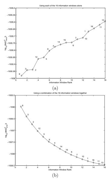
**Fig. 5.5**: Graphs of the data contained in each Information Window versus the window rank when using (a) Simple Search and (b) Combinatorial Search. The numbers along the graph line are the window numbers.
