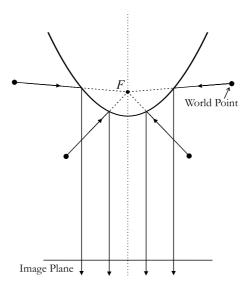
Fig. 2.5: Schematic of a Parabolic Mirror.
