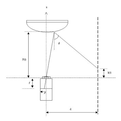
Fig. 2.15: Geometry of image formation using a catadioptric sensor with a constant vertical resolution mirror profile.
