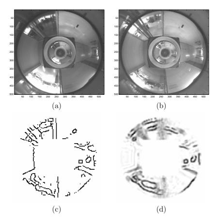
Fig. 4.12: (a) An omnidirectional image obtained at 11 am, (b) one obtained at 5 pm (c) An edge-detected image and (d) its retrieved image.
