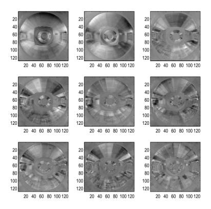
${f Fig.~3.5}$ : The first 9 (omnidirectional) eigenimages obtained via Principal Component Analysis.
