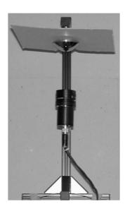
Fig. 2.13: The SVAVISCA omnidirectional camera with a specialised mirror
