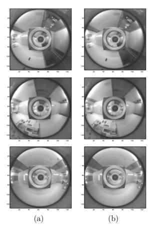
Fig. 3.6: IST Set: A selection of (a)omnidirectional test images and (b) their closest matches obtained by projection into a 10D eigenspace. The *a priori* inter-image distance was 20 cm and each image was  $128 \times 128$  pixels in size.
