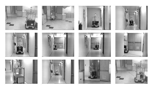
**Fig. 4.9**: A sequence of images of an experiment combining Visual Path Following for door traversal and topological navigation for corridor following.
