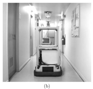
**Fig. 4.1**: (a) The omnidirectional camera with a spherical mirror and (b) the camera mounted on a Labmate mobile platform.
