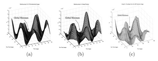
**Fig. 5.12**: Graphs showing images acquired at run-time versus those acquired a priori when using (a)  $16 \times 16$  Omnidirectional Images, (b)  $4 \times 4$  Information Windows and (c)  $8 \times 10$  Information Windows. Experiments were undertaken along a  $\sim 7$ m path.
