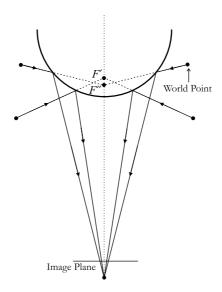
Fig. 2.7: Schematic of a Spherical Mirror.
