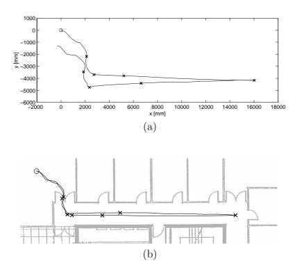
Fig. 4.10: The experiment combining Visual Path Following for door traversal and topological navigation for travelling long distances. Trajectory estimate from (a) odometry and (b) the true trajectory.
