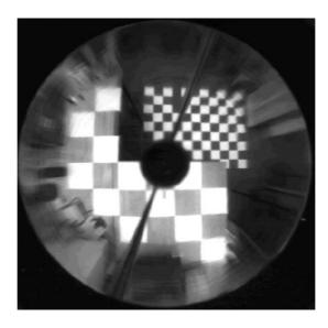
**Fig. 2.9**: Hicks and Bajcsy designed a mirror which approximates a perspective projection. In this case, two orthographic views of the ground plane are correctly mapped from the *same* mirror (from [59]).
