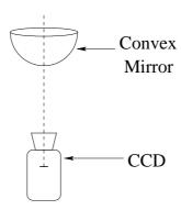
Fig. 1.5: Schematic of an omnidirectional system with a standard convex mirror.
