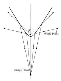
Fig. 2.6: Schematic of a Hyperbolic Mirror.
