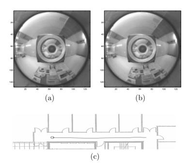
**Fig. 5.9**: (a) An unknown image, (b) its closest match and (c) the path travelled by the robot when using entire  $128 \times 128$  images.
