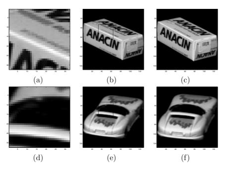
**Fig. 5.15**: Object recognition and pose estimation without background variation. When using the *most* discriminating Information Window, the object recognition rate was 95.3% and the pose estimation rate 73.8%.
