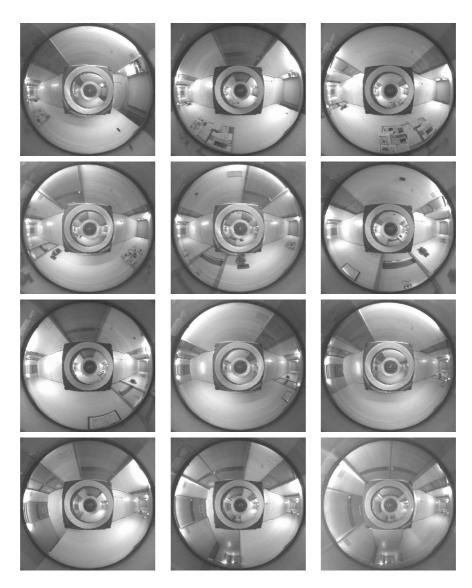
**Fig. 3.2**: A sequence, from left-to-right and top-to-bottom, of omnidirectional images acquired along a corridor at a full resolution of  $516 \times 508$  pixels. Before applying Principal Component Analysis, these were reduced to a resolution of  $128 \times 128$  pixels.
