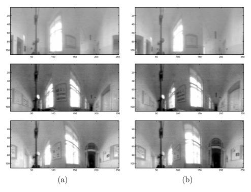
**Fig. 3.7**: CMP Set: A selection of (a) panoramic test images and (b) their closest matches obtained by projection into a 10D eigenspace. The *a priori* inter-image distance was 50cm and each image was  $252 \times 110$  pixels in size.
