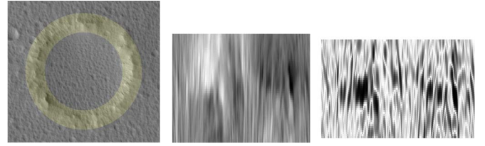
Fig. 1. Image transformation. (Left) Original image and sampling points, (center) polar image, and (right) edge map.
