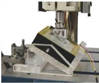
Fig. 5. The addition of the adjustable angle tilt stage and the angled push plate. The figure shows the 30-degree setup where the stage is adjusted to 30 degrees and the 30-degree push plate is used.
