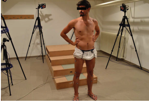
Fig. 3. Experimental setup: The subject with the marker placement and the stairs
