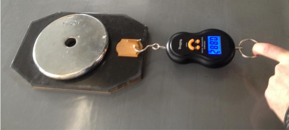
Fig. 3.11 Coefficient of friction measurement. We estimate the COF of a material by several measurements of the maximum friction force on the robot foot, loaded with a 1.5kg mass.
