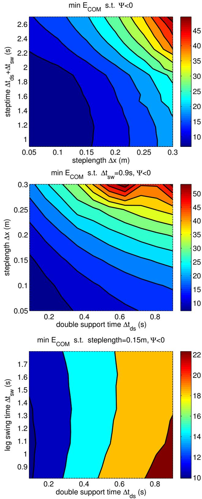
Fig. 2.4 Minimum  $E_{COM}$  on flat terrain, measured in physics simulation.
