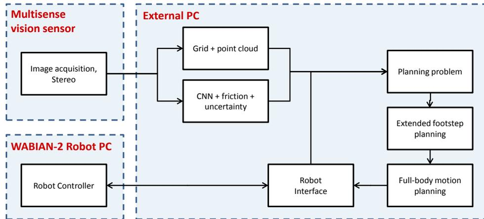
Fig. 5.1 System architecture
