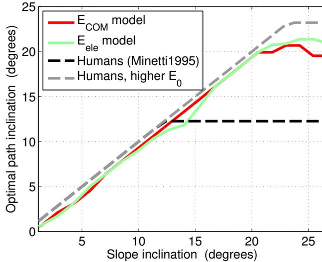
Fig. 2.9 Optimal path inclination angle  $\alpha_{\text{path}}$  as a function of the slope angle  $\alpha$ . If  $\alpha_{\text{path}} < \alpha$  then the path is curved at shallower inclination and longer total distance.
