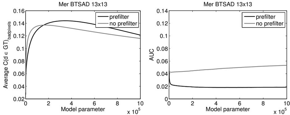
Fig. 4.5 Performance of models with parameter values changes with prefiltering conditions. Results obtained from the Cones image of the indoors set.
