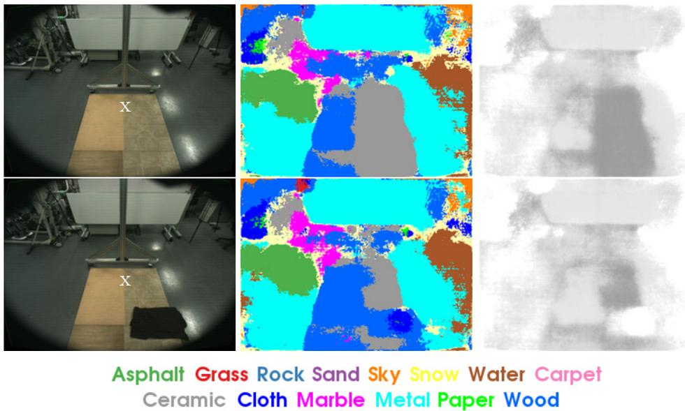
Fig. 5.2 Mock-up scenario and friction from vision. Left: the view from the robot’s camera of the mock-up scenario built in the laboratory. The locomotion target is one meter ahead, marked with a white “x”. Middle: material segmentation. Right: coefficient of friction quantiles  $Q_{1-0.95}$  of equation (3.9). Darker shades of gray correspond to higher friction, such that white is  $\mu = 0$  and black  $\mu = 1$ .
