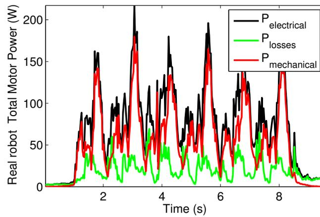
Fig. 2.11 Real total electrical power measured over a 6-step trial.
