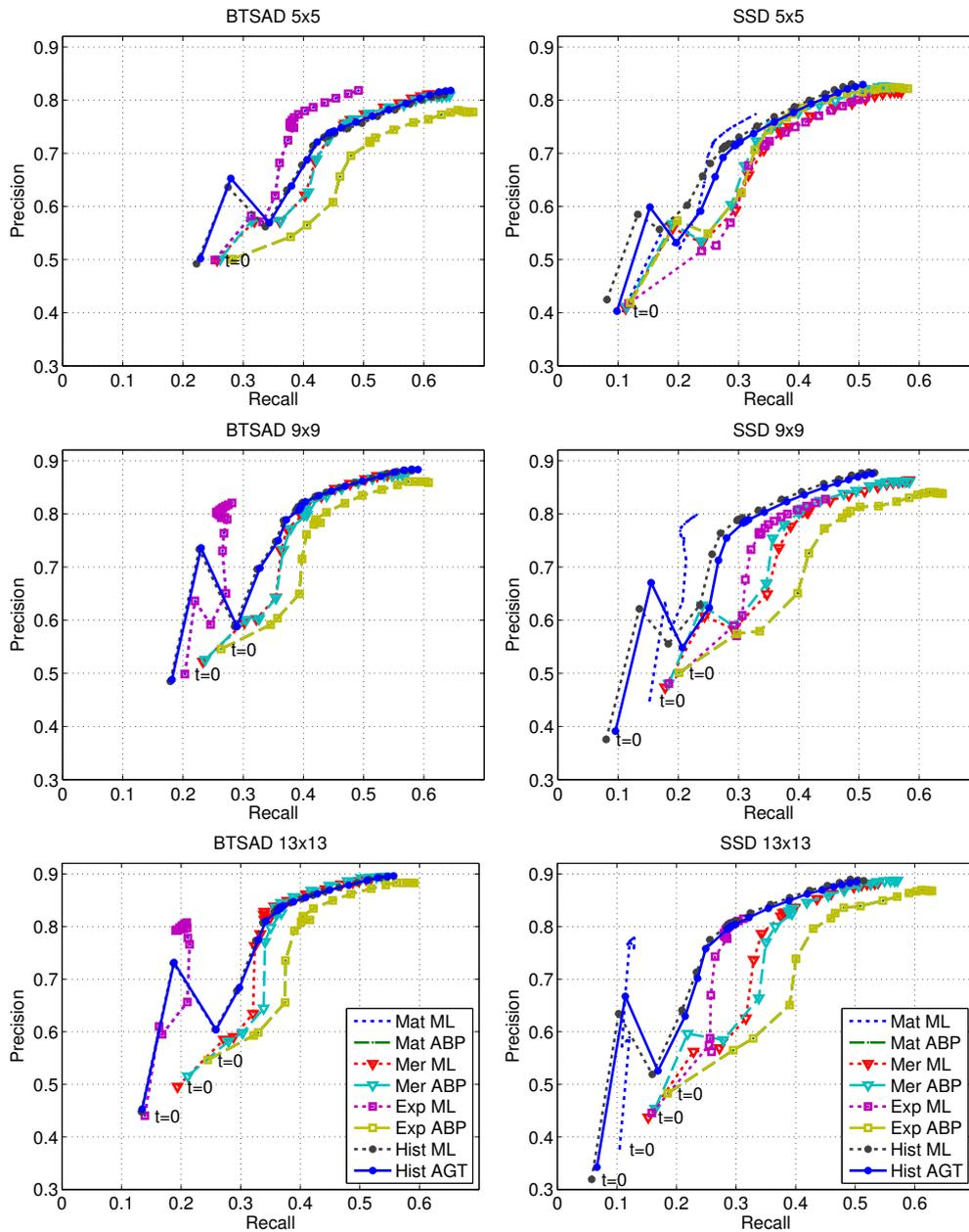
Fig. 4.10 Comparison of the performance of all models along time when used with the occupancy grid algorithm. Each point represents a different instant of time, while the first frame of the image sequence is marked with  $t=0$ . “Mat ABP” overlaps perfectly with “Exp ABP” on both cost functions, and “Mat ML” overlaps perfectly with “Exp ML” for the BTSAD cost function.
