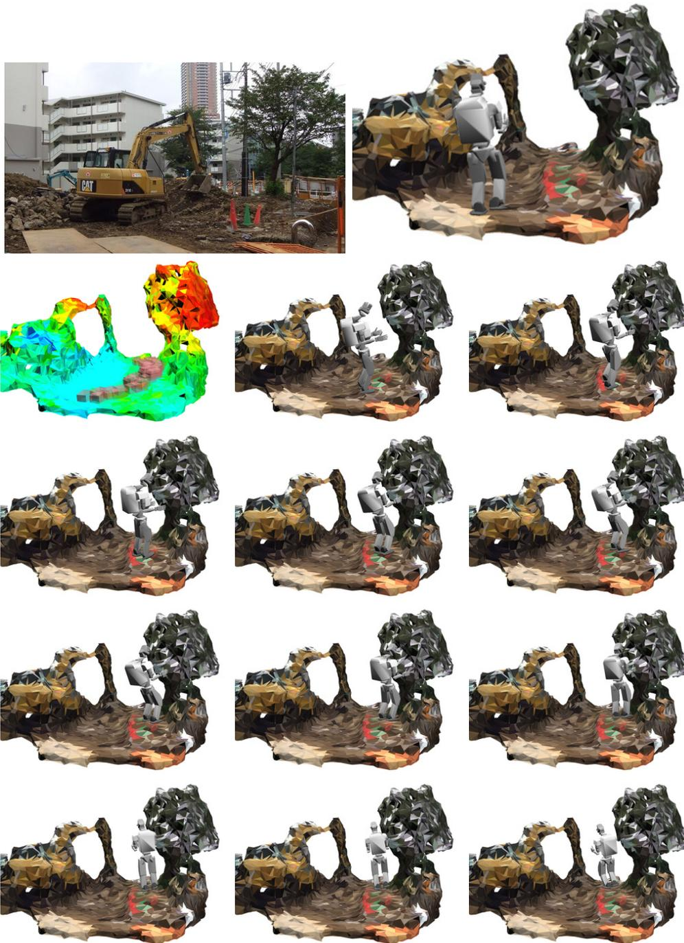
Fig. 5.5 Simulation results on real stereo data. In order: original picture, 3D-reconstructed scenario together with initial pose, friction-colored scenario together with footstep plan, image sequence of planned trajectory. Friction coloring: cold colors are high friction and warm are low (i.e. red is  $\mu = 0$ , blue  $\mu = 1$ ).
