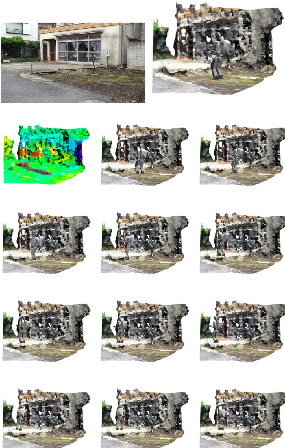
Fig. 5.7 Simulation results on real stereo data. In order: original picture, 3D-reconstructed scenario together with initial pose, friction-colored scenario together with footstep plan, image sequence of planned trajectory. Friction coloring: cold colors are high friction and warm are low (i.e. red is  $\mu = 0$ , blue  $\mu = 1$ ).
