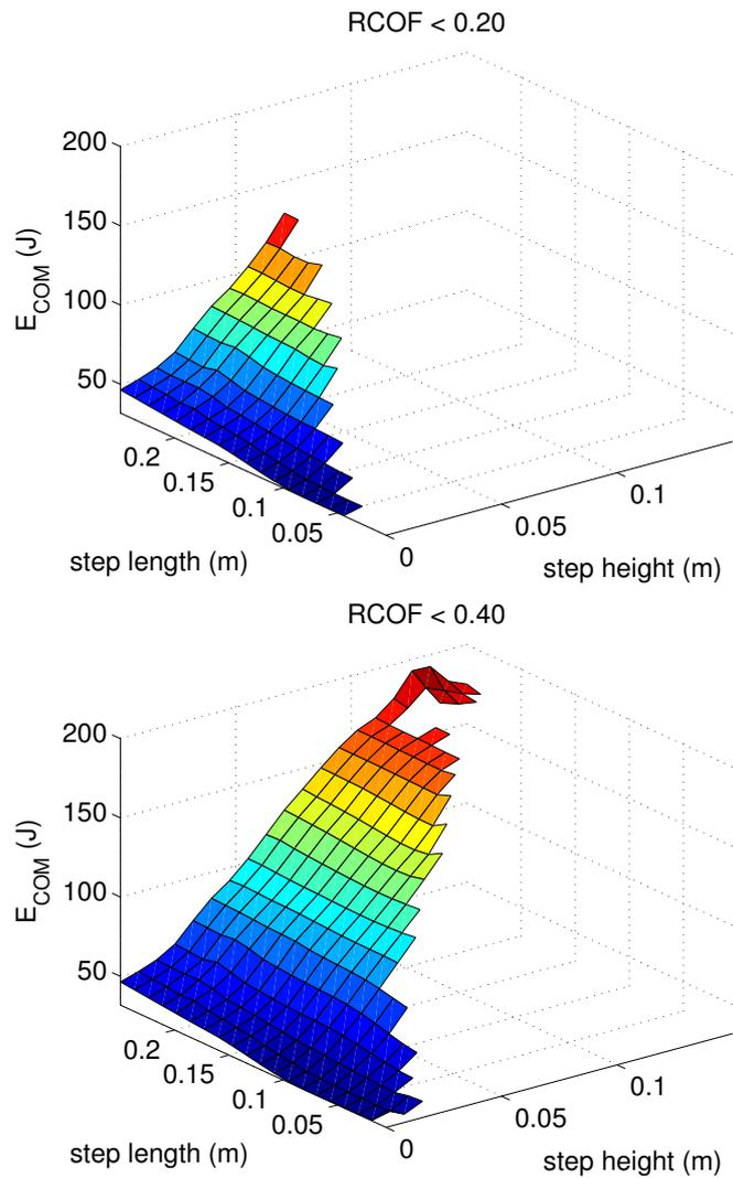
Fig. 2.3 Minimum  $E_{COM}$  on slopes, as a function of step length and step height. Measured in physics simulation.
