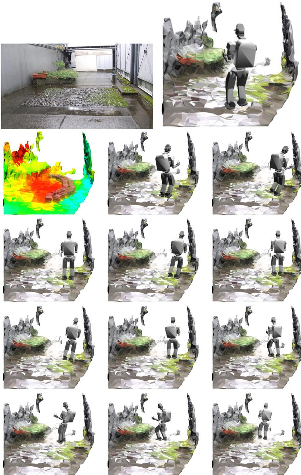
Fig. 5.9 Simulation results on real stereo data. In order: original picture, 3D-reconstructed scenario together with initial pose, friction-colored scenario together with footstep plan, image sequence of planned trajectory. Friction coloring: cold colors are high friction and warm are low (i.e. red is  $\mu = 0$ , blue  $\mu = 1$ ).
