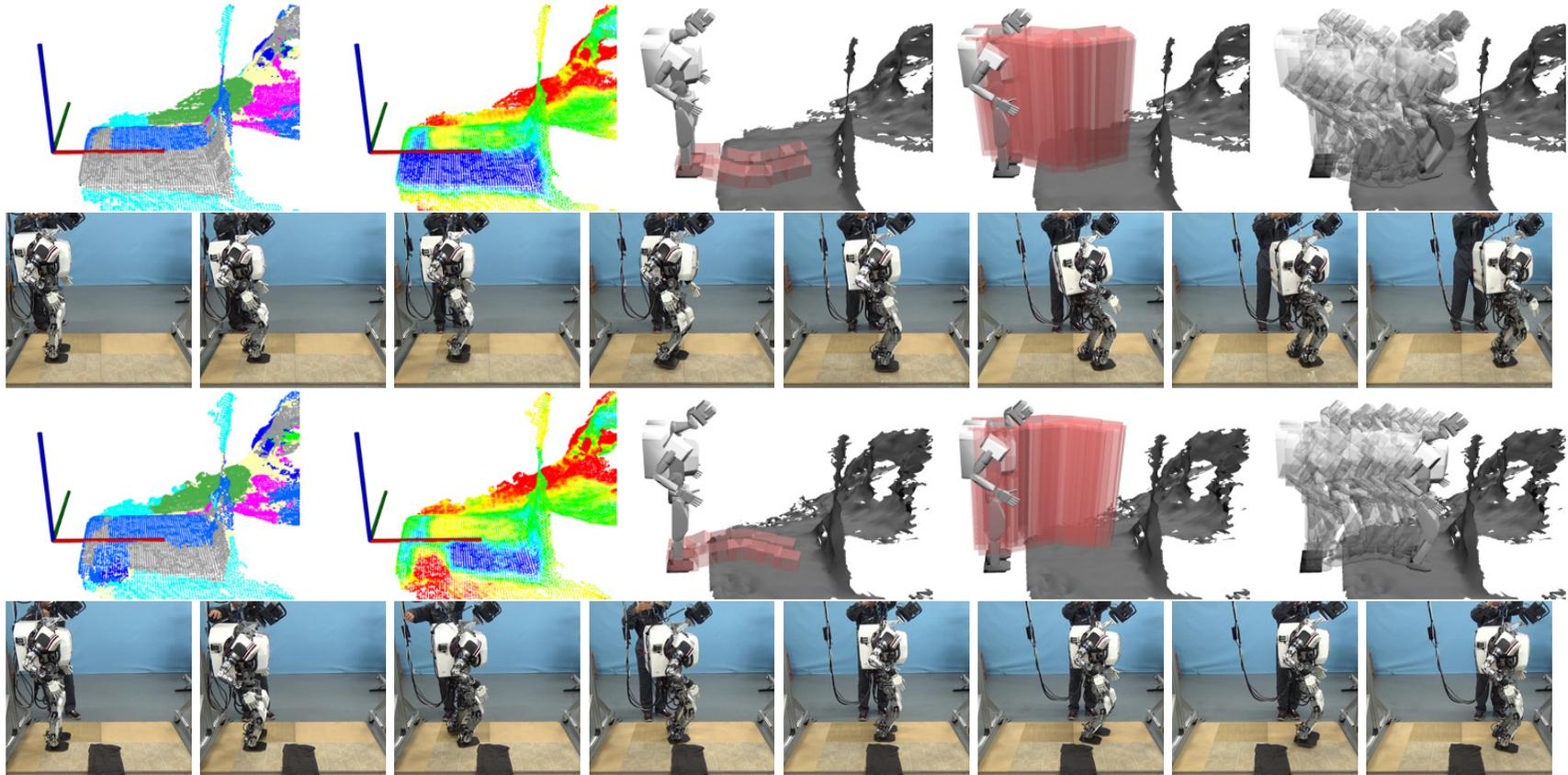
Fig. 5.3 Perception, planning and locomotion results on the mock-up scenario. First two rows: two surfaces (wood and ceramic).
