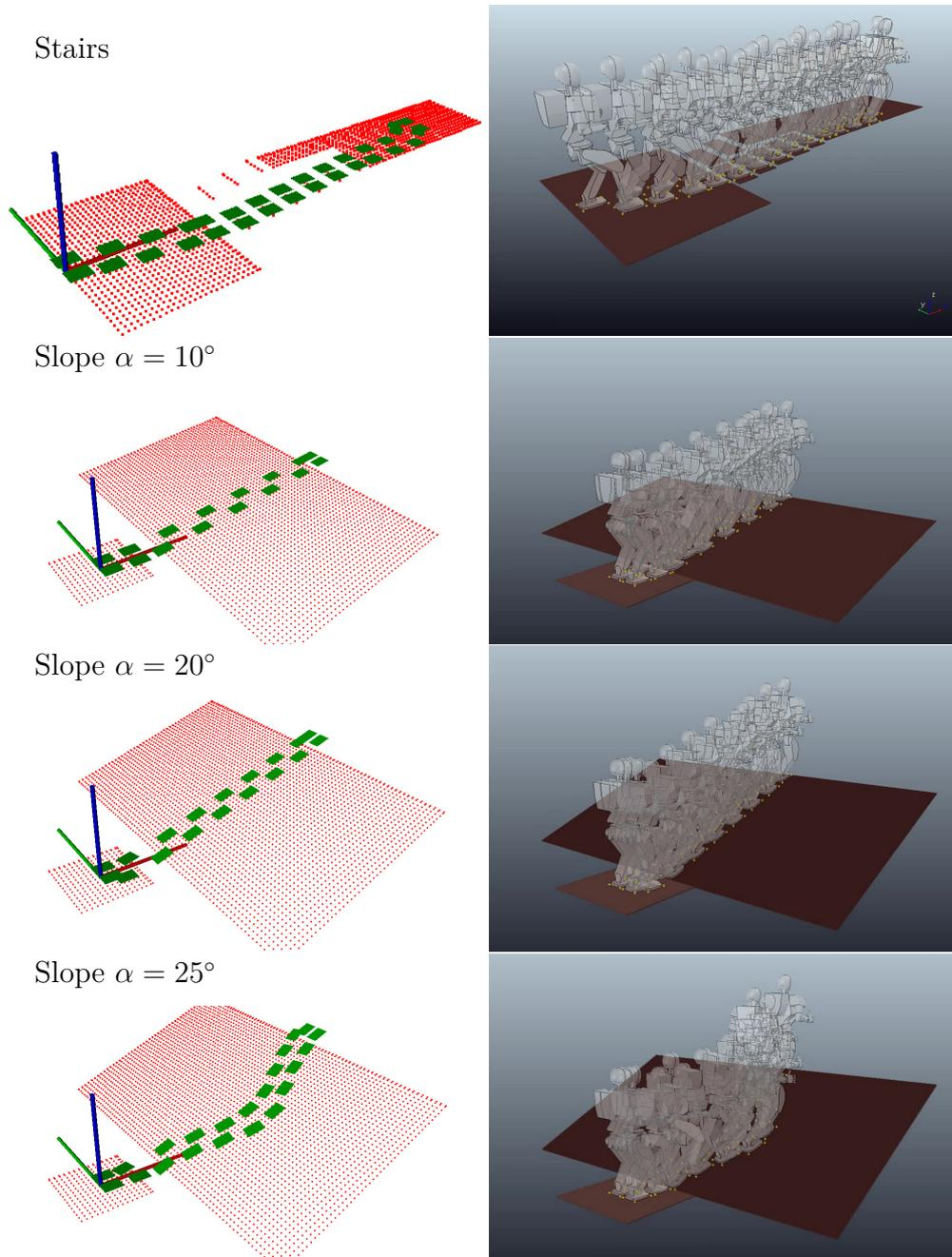
Fig. 2.8 Optimal plans obtained by our planner in the “Stairs” and “Slope” scenarios. On steep stairs and slopes, it is more energy optimal to walk a longer inclined distance but at a lower angle.
