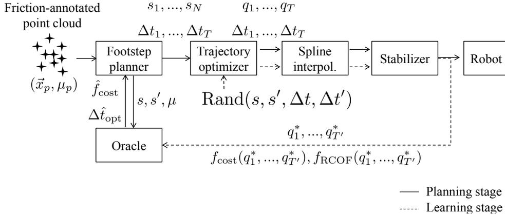
Fig. 2.13 Our hierarchical planning architecture, which uses trajectory optimization to minimize a cost function  $f_{\text{cost}}$ , as well as oracle costs to plan footstep placement and timing that will have low predicted  $f_{\text{cost}}$ .
