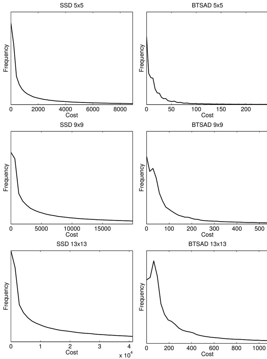
Fig. 4.2 Distribution of costs at true disparity ( $E_{1,d^*}$ ) for SSD (left) and BTSAD (right) cost functions on a 5x5, 9x9 and 13x13 window. Horizontal axis represents the values of  $E_{1,d^*}$ .
