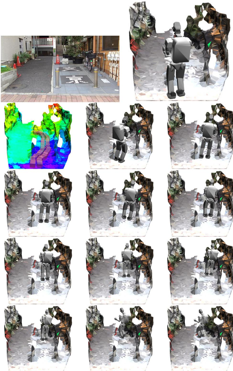
Fig. 5.8 Simulation results on real stereo data. In order: original picture, 3D-reconstructed scenario together with initial pose, friction-colored scenario together with footstep plan, image sequence of planned trajectory. Friction coloring: cold colors are high friction and warm are low (i.e. red is  $\mu = 0$ , blue  $\mu = 1$ ).
