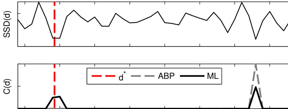
Fig. 4.6 Confidence  $C(d)$  using Merrell’s model with ABP and ML parameters. Dashed red line indicates true disparity  $d^*$  as indicated by the dataset. Results taken from pixel (364,150) of the Teddy image, as an example of ML’s better performance seen in Table 4.2. ML does not require ground-truth and leads here to higher  $C(d^*)$ .
