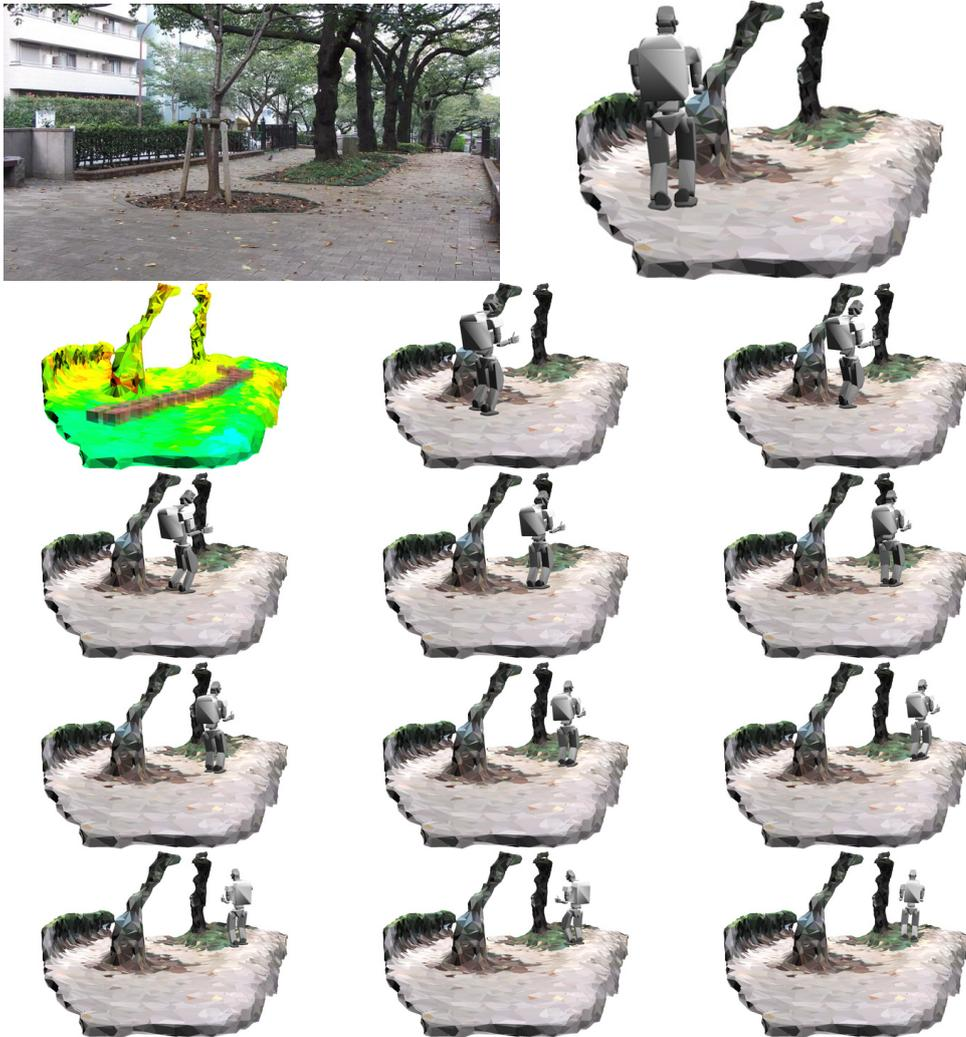
Fig. 5.4 Simulation results on real stereo data. In order: original picture, 3D-reconstructed scenario together with initial pose, friction-colored scenario together with footstep plan, image sequence of planned trajectory. Friction coloring: cold colors are high friction and warm are low (i.e. red is  $\mu = 0$ , blue  $\mu = 1$ ).
