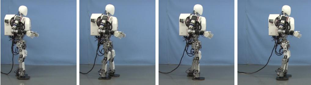
Fig. 2.10 Real robot walking with  $E_{\text{COM}}$ -optimal parameters (red dot in Figure 2.12).
