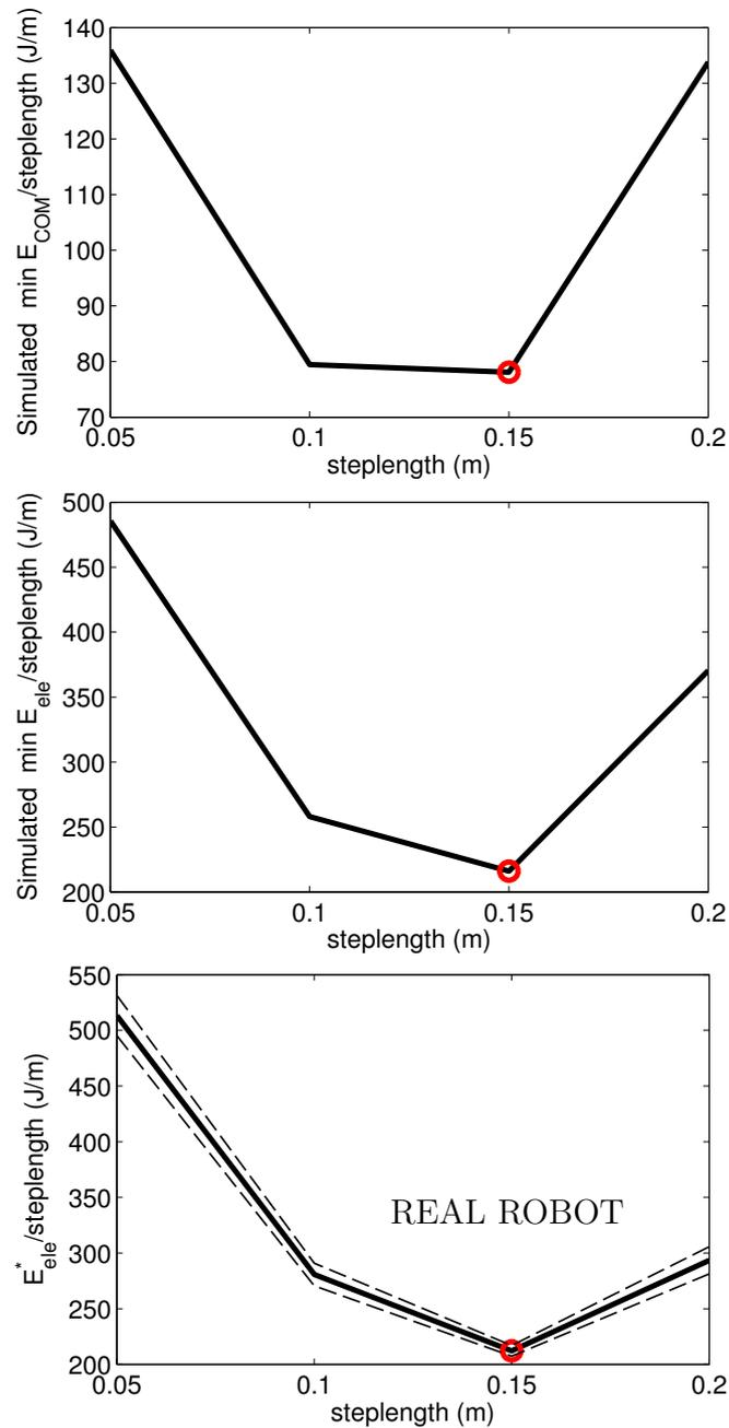
Fig. 2.12 Simulated versus real energy consumption. Mechanical energy  $E_{COM}$  (left), simulated electrical energy  $E_{ele}$  (middle) and measured electrical energy  $E_{ele}^*$  (right). The real energy curve was obtained by averaging over 18 steps for each step-length and standard deviation is also shown.
