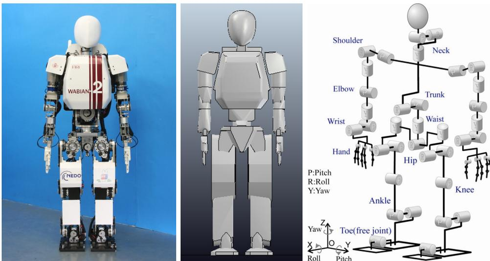
Fig. 2.1 The humanoid robot WABIAN-2, used in our simulation experiments. From left to right: real robot, simulated, DOF.
