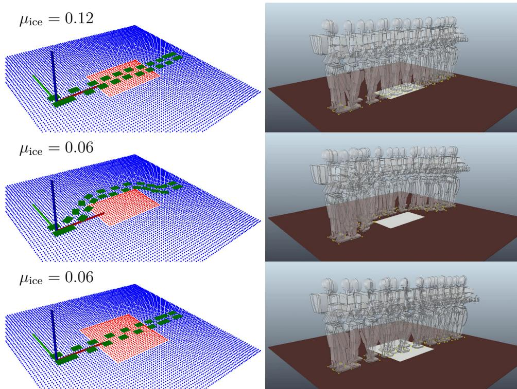
Fig. 2.7 Optimal plans obtained by our planner in the “ground and ice-patch” scenario. The top row shows the footstep plan and point cloud (red has friction  $\mu_{ice}$ , blue  $\mu_{ground} = 1$ ). Left: robot crosses a narrow ice patch ( $\mu_{ice} = 0.12$ ). Middle: robot walks around the patch if its slipperiness is increased ( $\mu_{ice} = 0.06$ ). Right: robot walks slowly through the same ice patch in case the ice is wider (energy spent avoiding it would be too high).
