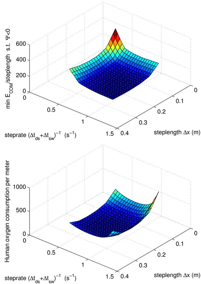
Fig. 2.6 Comparison of our robot's and humans' cost of transport. Top: Our robot's minimum  $E_{\text{COM}}$  per distance travelled. Bottom: Oxygen consumption of a human with WABIAN-2's physical limits, given by the empirical formulas of human walking of [81]. Units are in percentage of the minimum.
