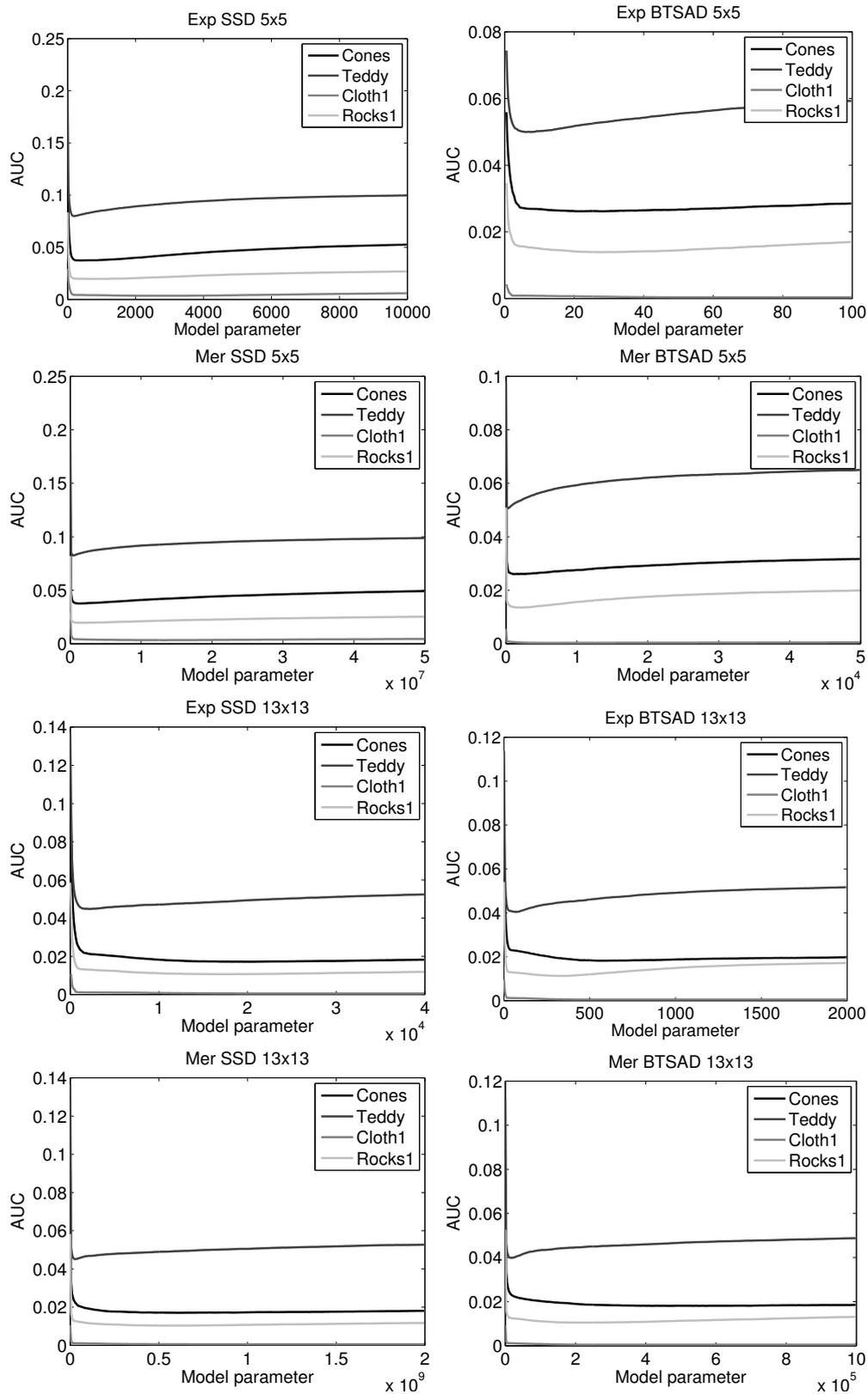
Fig. 4.4 The parametric models' cliff-maximum-and-tail of performance (AUC). Results with the different cost functions and window sizes are shown. Note how the curves and optimal parameters vary both between images and cost functions. Figures for Matthies' model are not shown since they can be obtained by linearly rescaling the horizontal axis of the exponential model's figures (see equations (4.4), (4.5) and (4.7)).
