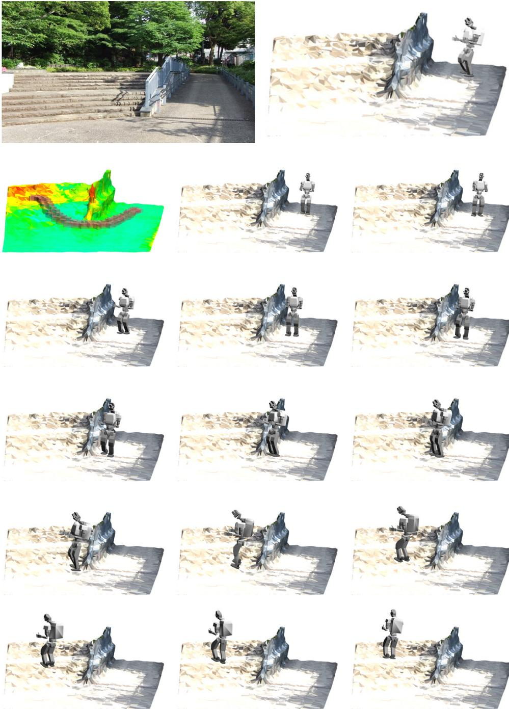
Fig. 5.6 Simulation results on real stereo data. In order: original picture, 3D-reconstructed scenario together with initial pose, friction-colored scenario together with footstep plan, image sequence of planned trajectory. Friction coloring: cold colors are high friction and warm are low (i.e. red is  $\mu = 0$ , blue  $\mu = 1$ ).
