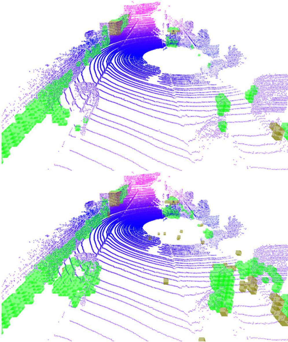
Fig. 4.11 Reconstruction results obtained using a BTSAD 13x13 cost function with the two top models. Top: Merrell's model. Bottom: HSM. Green squares represent true-positives (i.e. cells correctly classified as occupied), brown squares represent false-positives (i.e. cells incorrectly classified as occupied).
