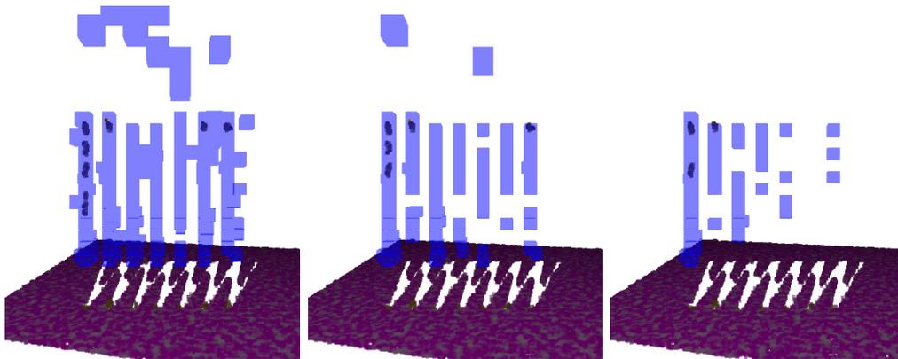
Fig. 4.8 Resulting occupancy grid computed in a traditional winner-take-all approach when using three different filtering thresholds (Peak Ratio). Left: 1.4. Center: 1.5. Right: 1.6. Occupied cells are marked with blue. The result should be 7 parallel bars.
