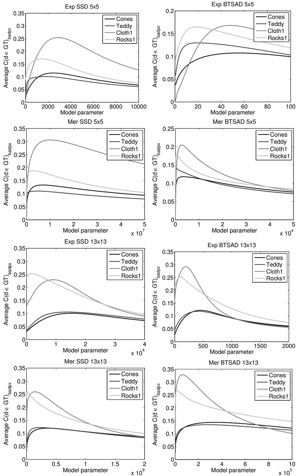
Fig. 4.3 The parametric models' cliff-maximum-and-tail of performance ( $C(d \in GT)_{badpx}$ ). Results with the different cost functions and window sizes are shown. Note how the curves and optimal parameters vary both between images and cost functions. Figures for Matthies' model are not shown since they can be obtained by linearly rescaling the horizontal axis of the exponential model's figures (see equations (4.4), (4.5) and (4.7)).
