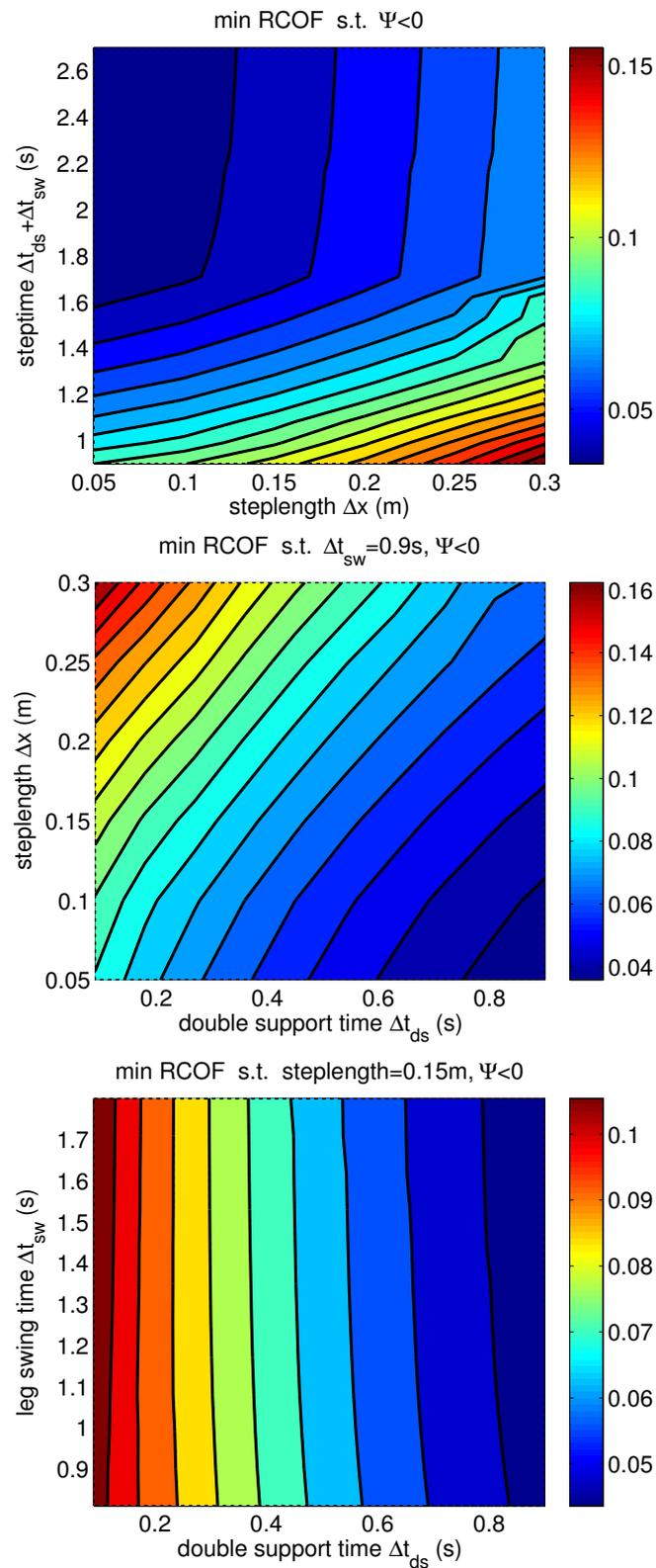
Fig. 2.5 Minimum RCOF on flat terrain, measured in physics simulation. RCOF is the maximum ratio of tangential-to-normal force over a step. It indicates the minimum ground coefficient of friction  $\mu$  where the robot can walk without slipping.
