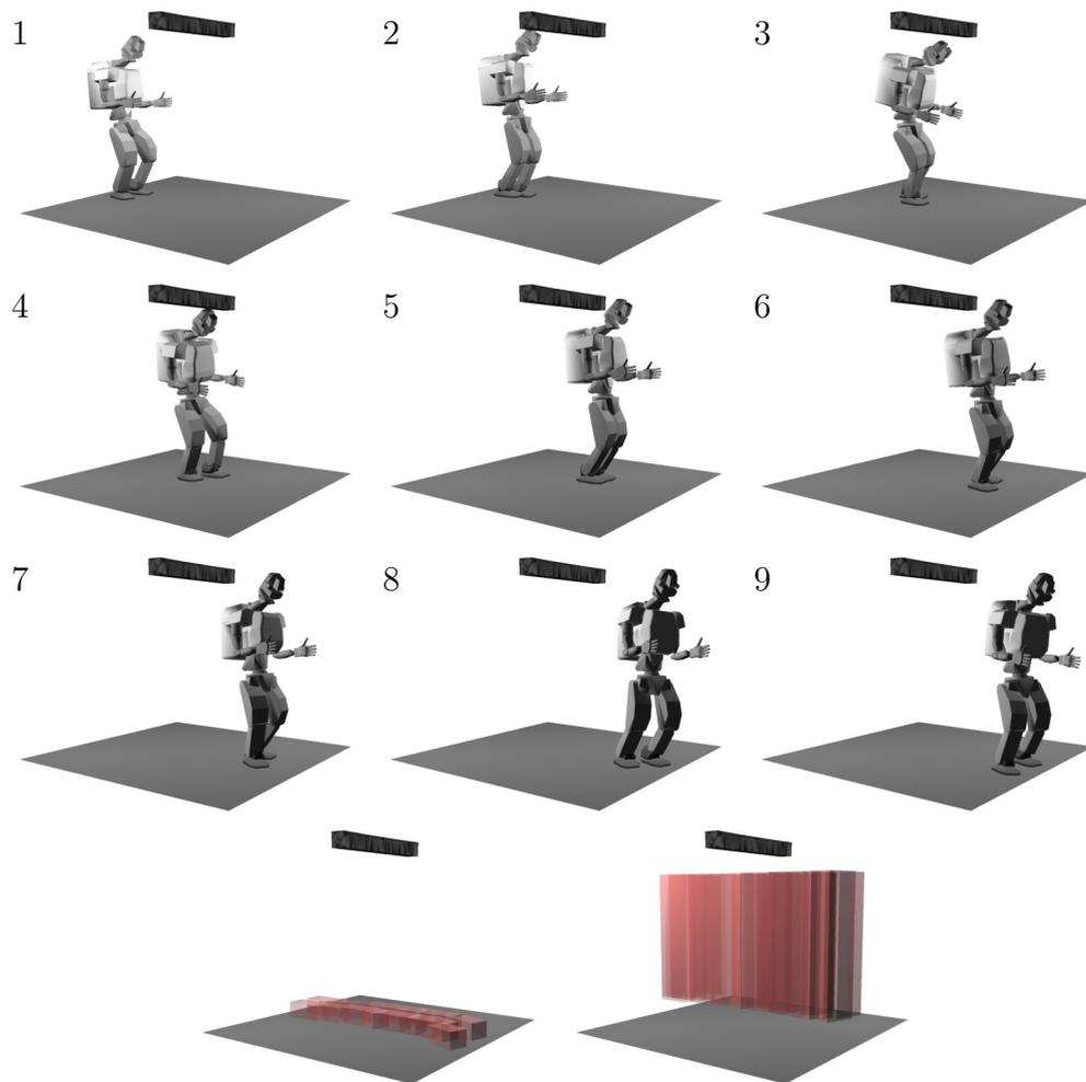
Fig. 2.14 Hierarchical locomotion planning with a high obstacle: walking sequence (1-9), footstep plan, and collision bounding boxes.
