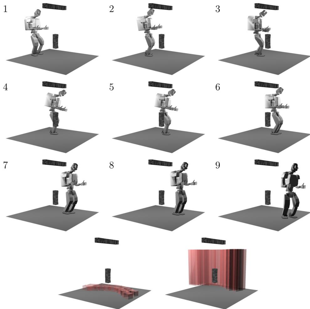
Fig. 2.15 Hierarchical locomotion planning with high and low obstacles: walking sequence (1-9), footstep plan, and collision bounding boxes.
