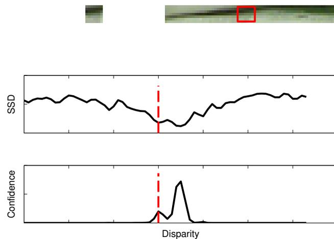
Fig. 4.1 Stereo matching confidence. Top: Matching a pixel in one image to pixels at different disparities in another image. Middle: Cost for each disparity. Bottom: Confidence measure computed from the cost values. Dashed line indicates true disparity. Even if the minimum cost is wrong, true disparity should still be attributed some confidence.
