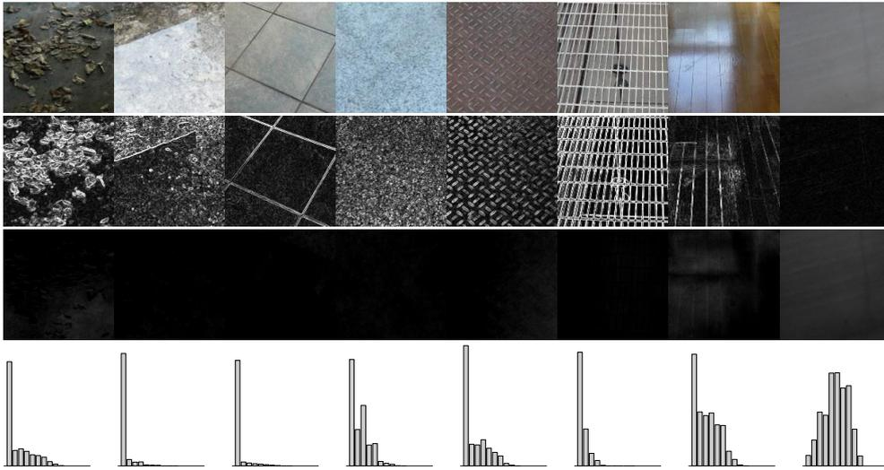
Fig. 3.9 Eight images from GTF sorted from lowest to highest COF. From top to bottom: original image, gradient image, shading image, histogram of shading image.
