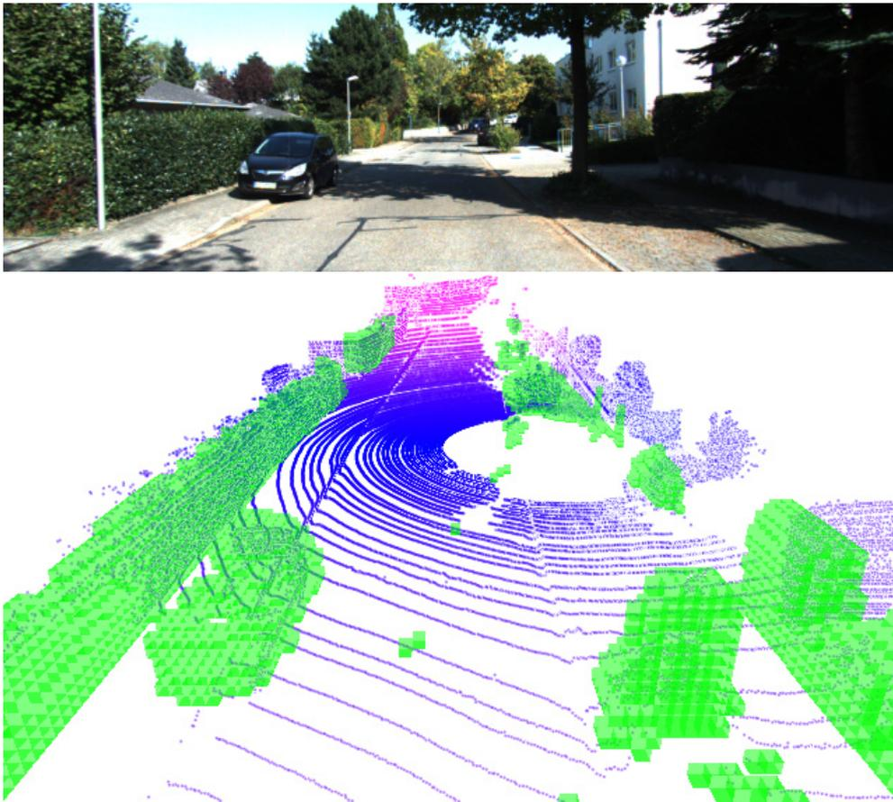
Fig. 4.9 The KITTI residential area dataset [185] used for occupancy grid evaluation. Green regions on the bottom image represent ground-truth occupied cells. Blue points represent laser data at one of the frames.
