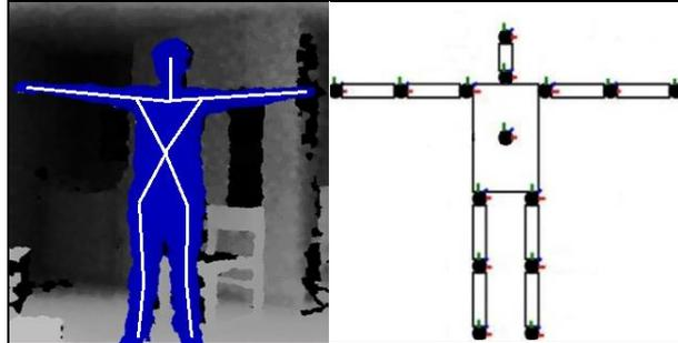
**Fig. 1** Skeleton tracking (left) and collected joints (right).
