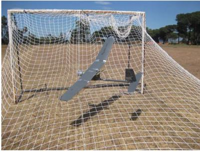
Fig. 16. Aircraft trapped in the retention system.
