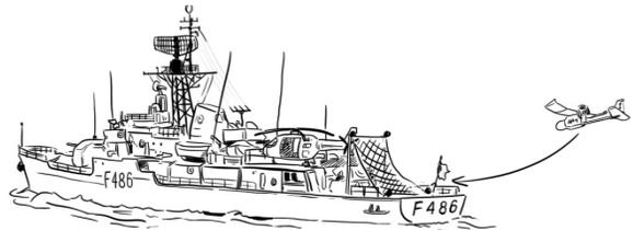
Fig. 1. Aircraft and naval platform with landmarks and restraint system.
